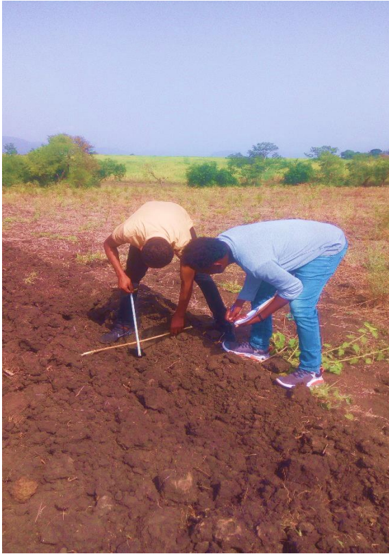
Annex 3. Depth and width of cut were measured by using tape metter.
