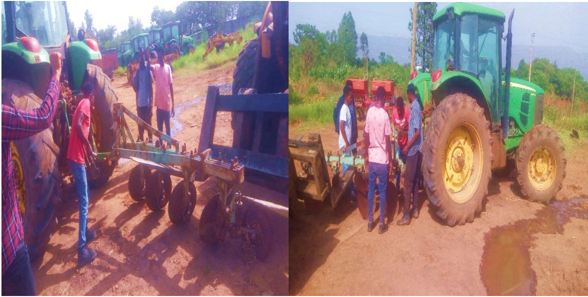
Annex1 Team of mechanics connecting and adjusting implement to tractor
