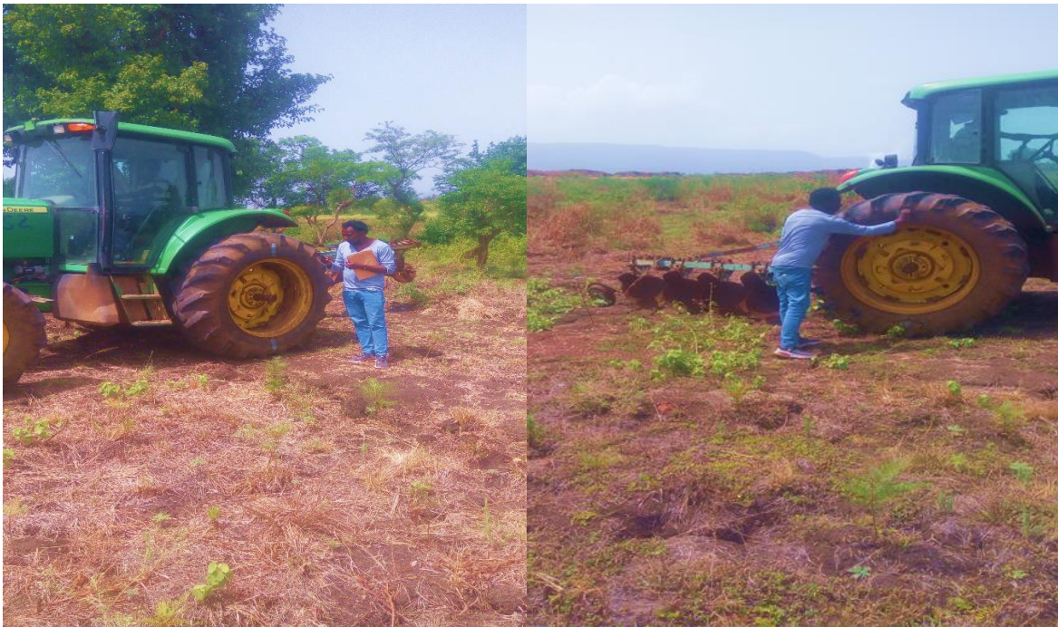
Annex 2. marking of tractor wheel for percentage evaluation of slippage.
