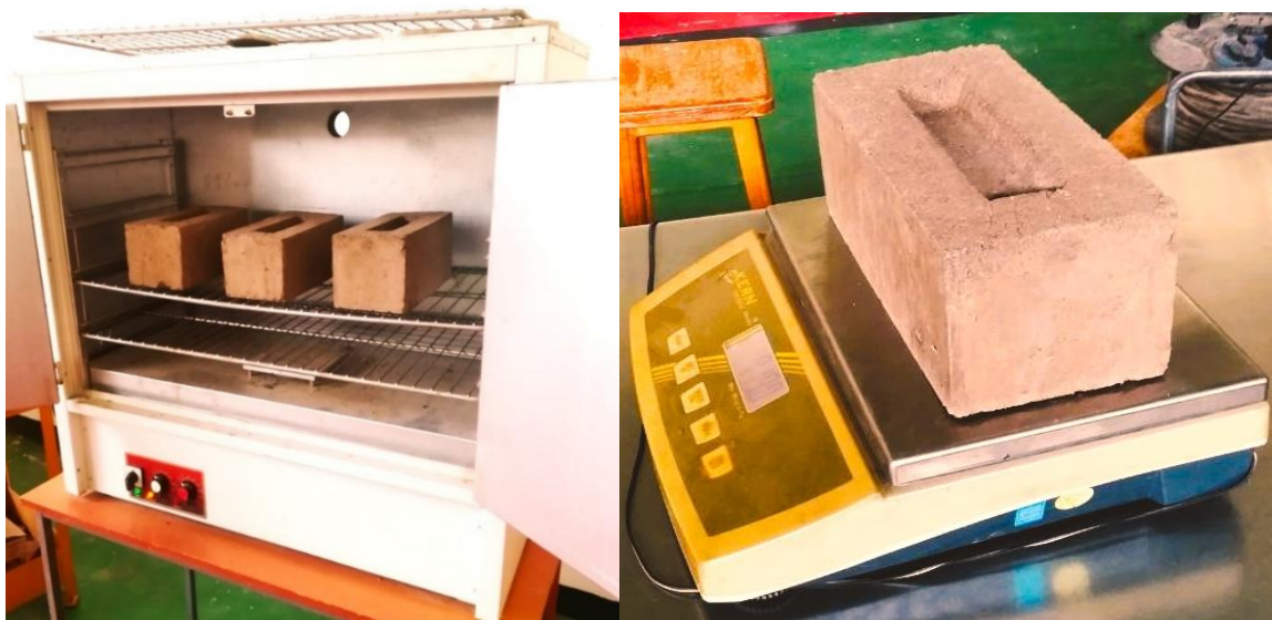
Figure 3.13: a) oven drying of soil blocks b) weighing soil blocks
