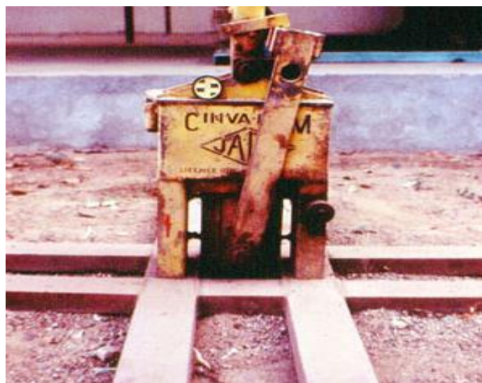
Figure 2.3: The first Manual press, CINVARAM (Shiferaw, 2008)
