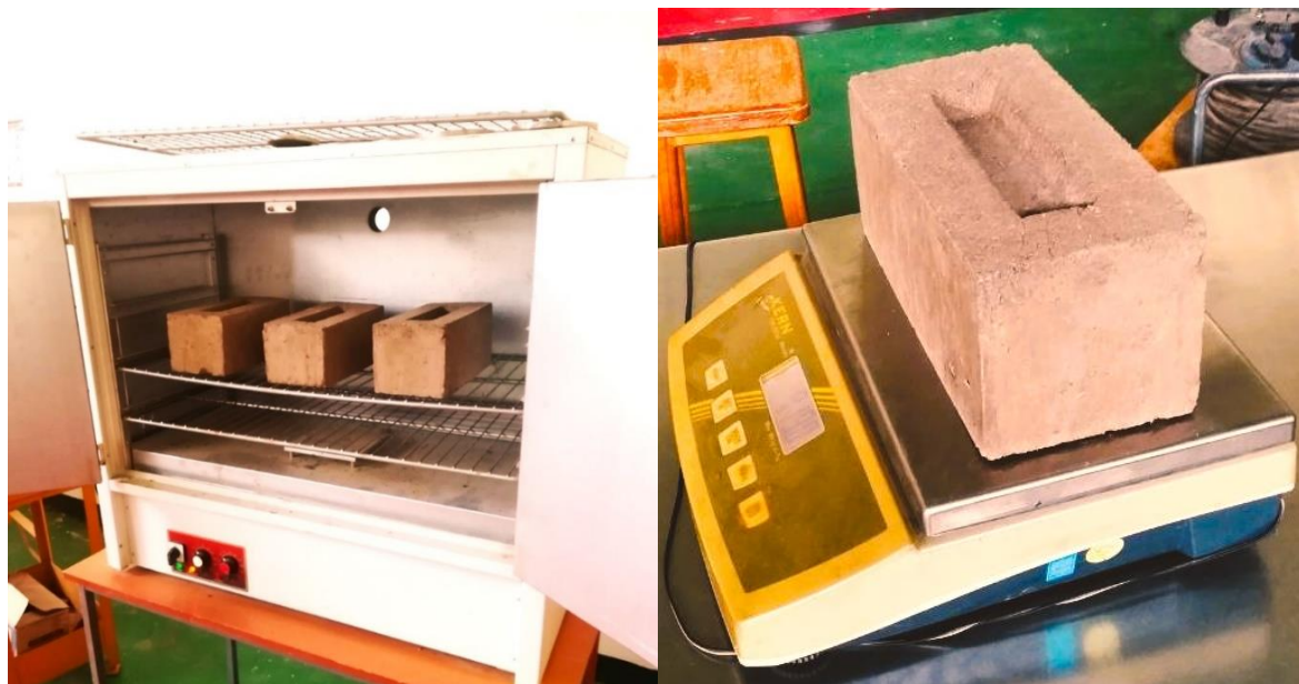
(c) Oven drying of sample & measuring for dry density test
