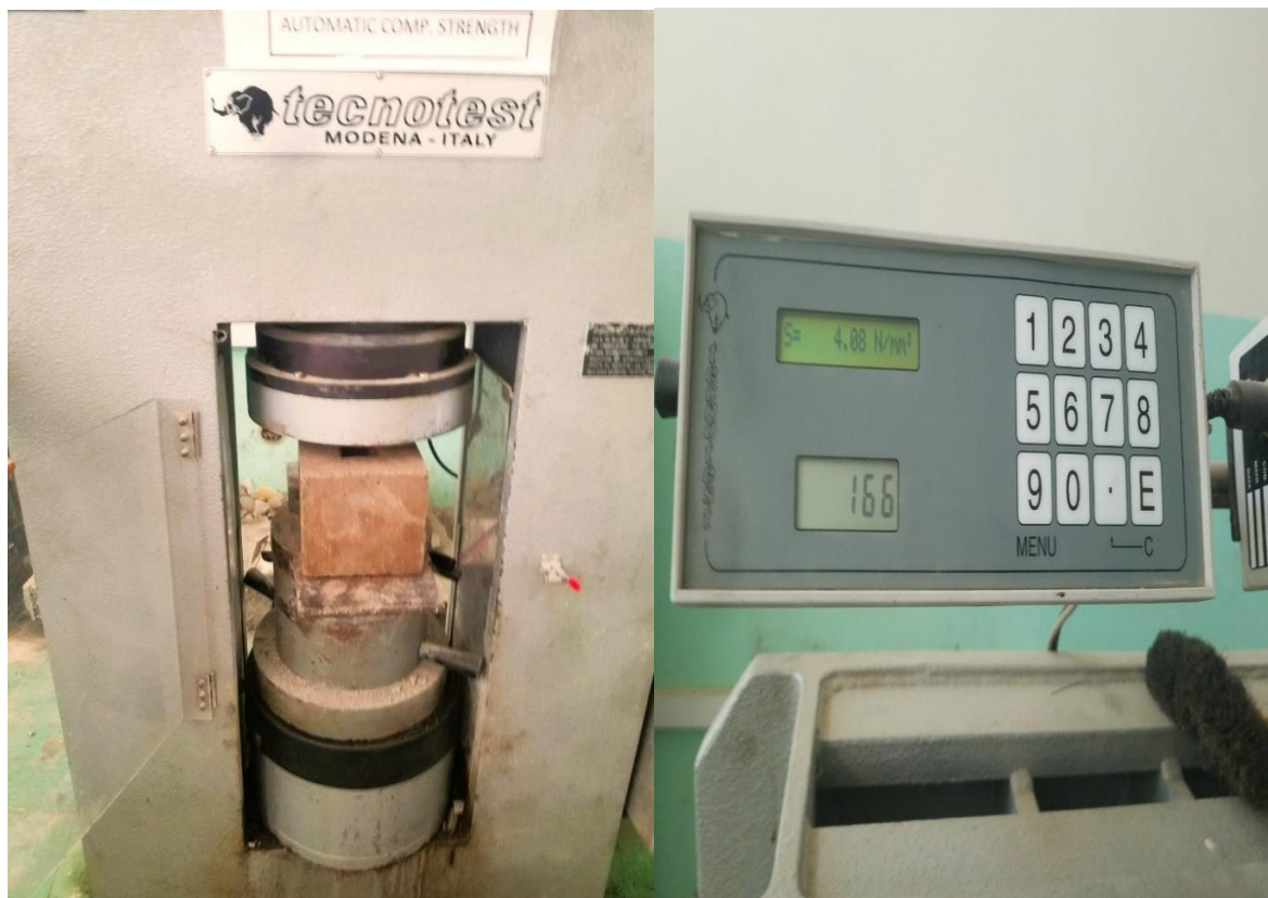
(b) Compressive strength test
