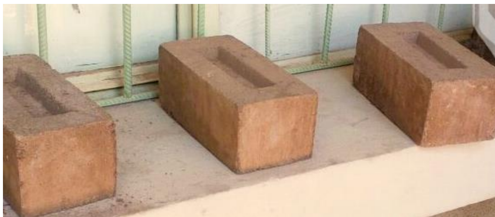
Figure 3.11: Stabilized soil blocks that have an average dimension of 290mm x 140mm x 100mm
