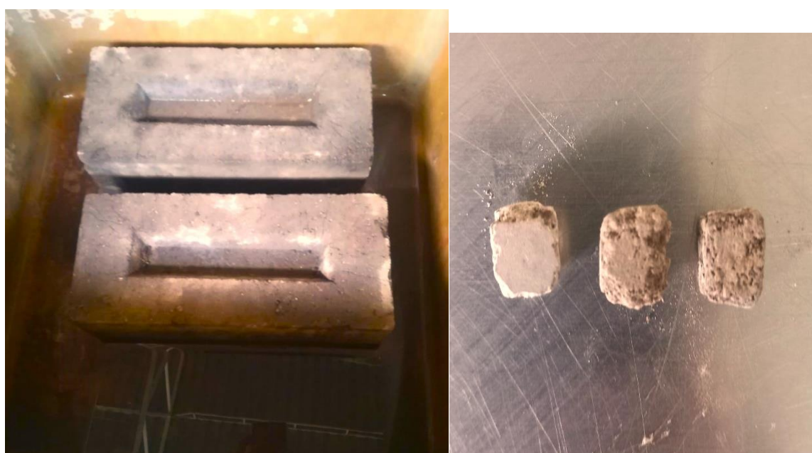
(d) Block preparation and water absorption test and Sample for SEM test
