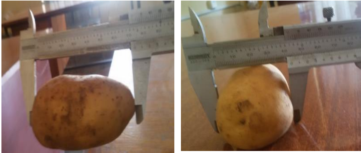
Figure 3. 2. Measuring potato size using caliper
