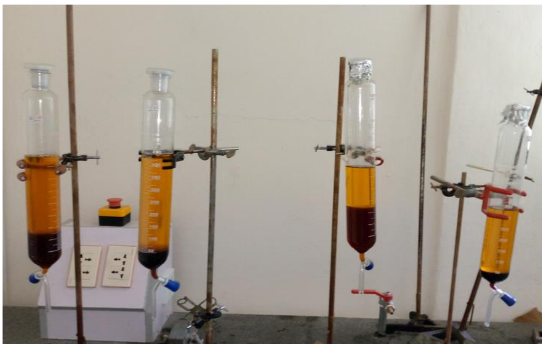
Figure 3.4 Glycerol and biodiesel separation in a separator funnel
