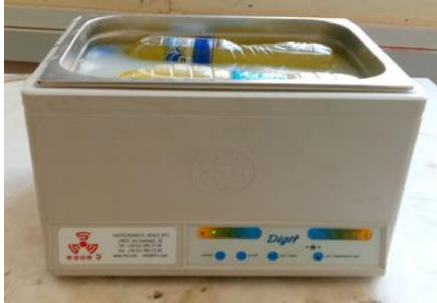
Figure 3.15 Photograph of the ultrasonicator used for mixing the fuel blends
