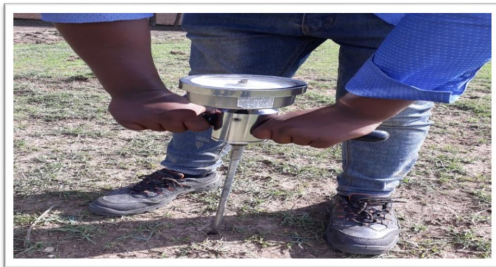
Fig. 3.4. Measuring soil resistance by cone penetrometer
