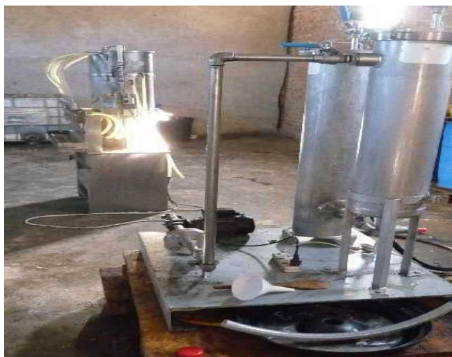
Figure 2. 4 Oil filtration machines for crude Jatropha oil
