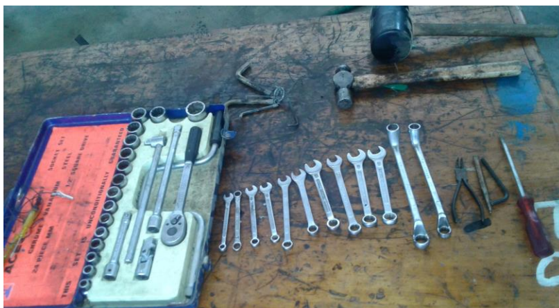
Figure 3. 12 Tools used for dismantling Robin DY-23 engine.
