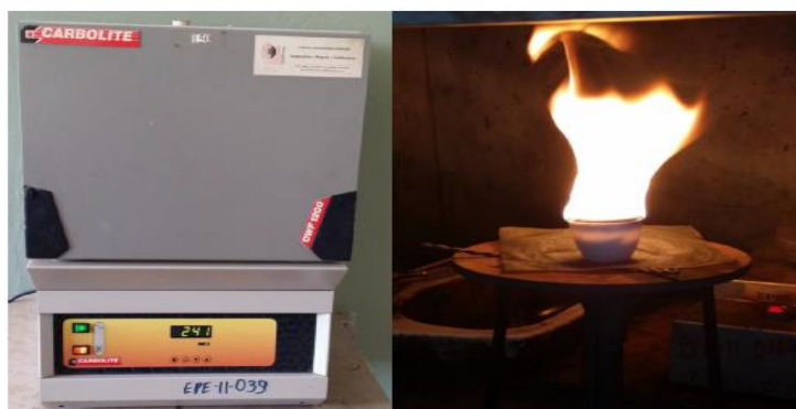
Figure 3. 10 Determination of ash content [24].
