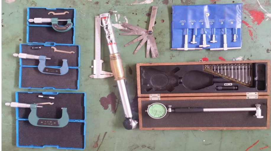
Figure 3. 13 Tools used for wear measures of the components.
