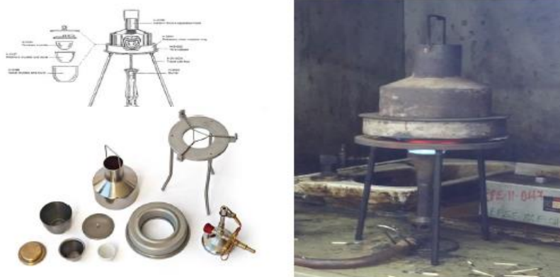
Figure 3. 11 Conoradson carbon residue determination [49].
