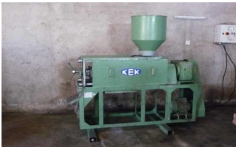
Figure 2. 5 Press machine for production of Jatropha oil used in Zambia
