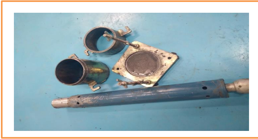
Figure 3.5 Compaction test equipment
