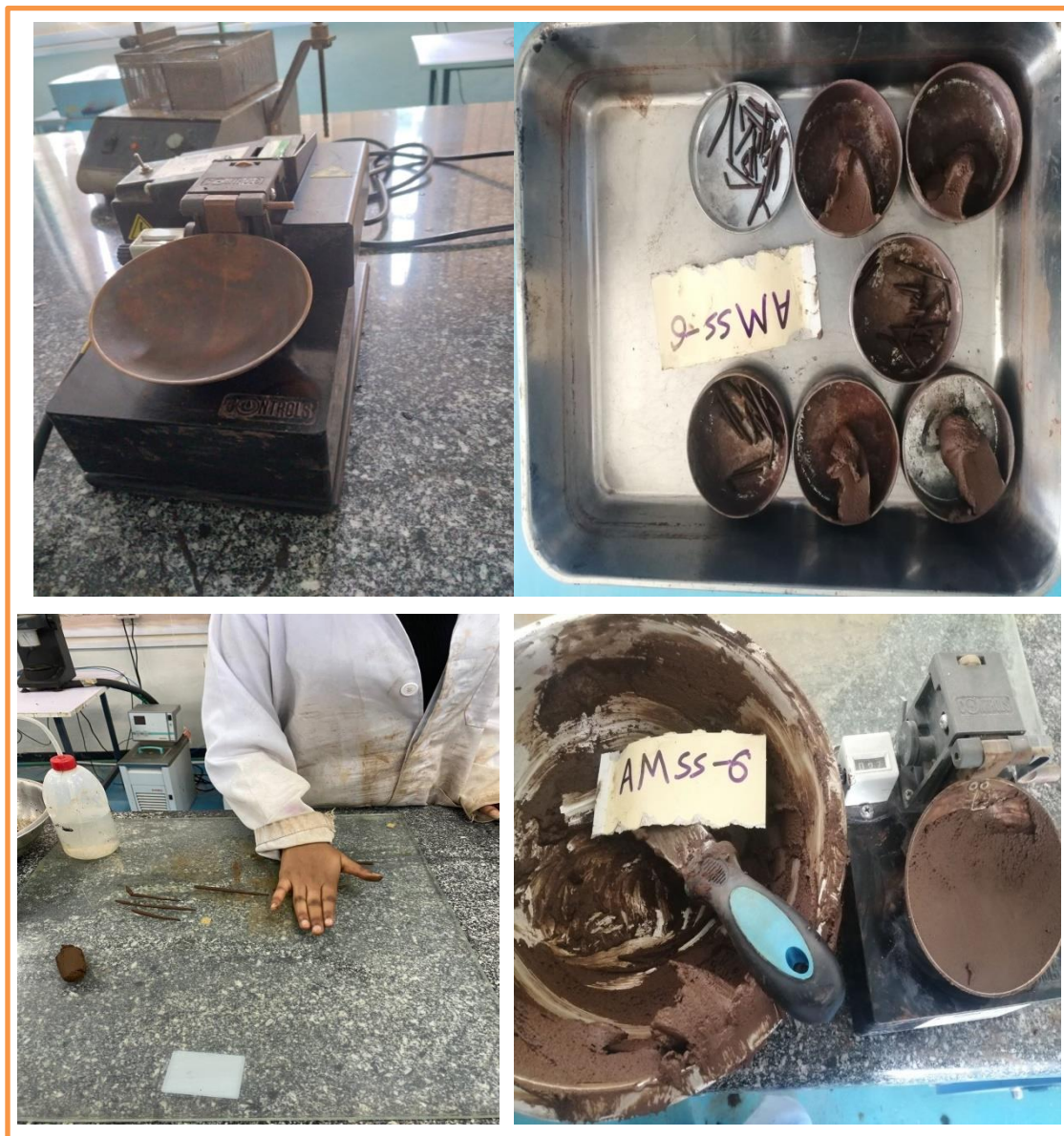
Figure 3.4 Methodology for Atterberg test
