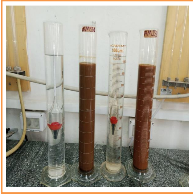
Figure 3.3 Hydrometer analysis, dispersed soil in 1000ml cylinder
