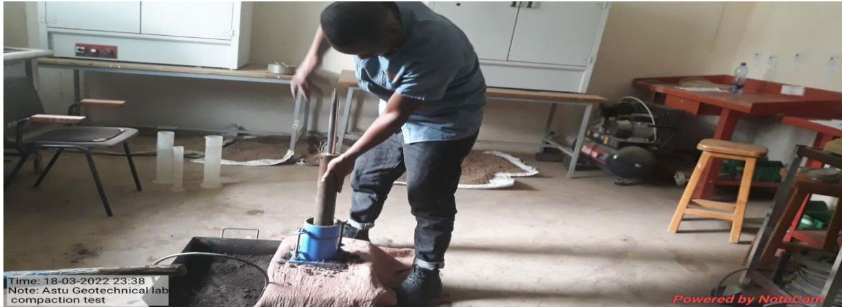
Figure 22: Standard compaction test
