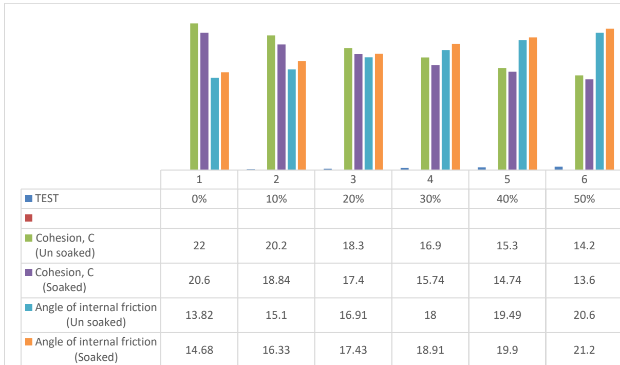
Figure 5.1 Direct Shear Tests
