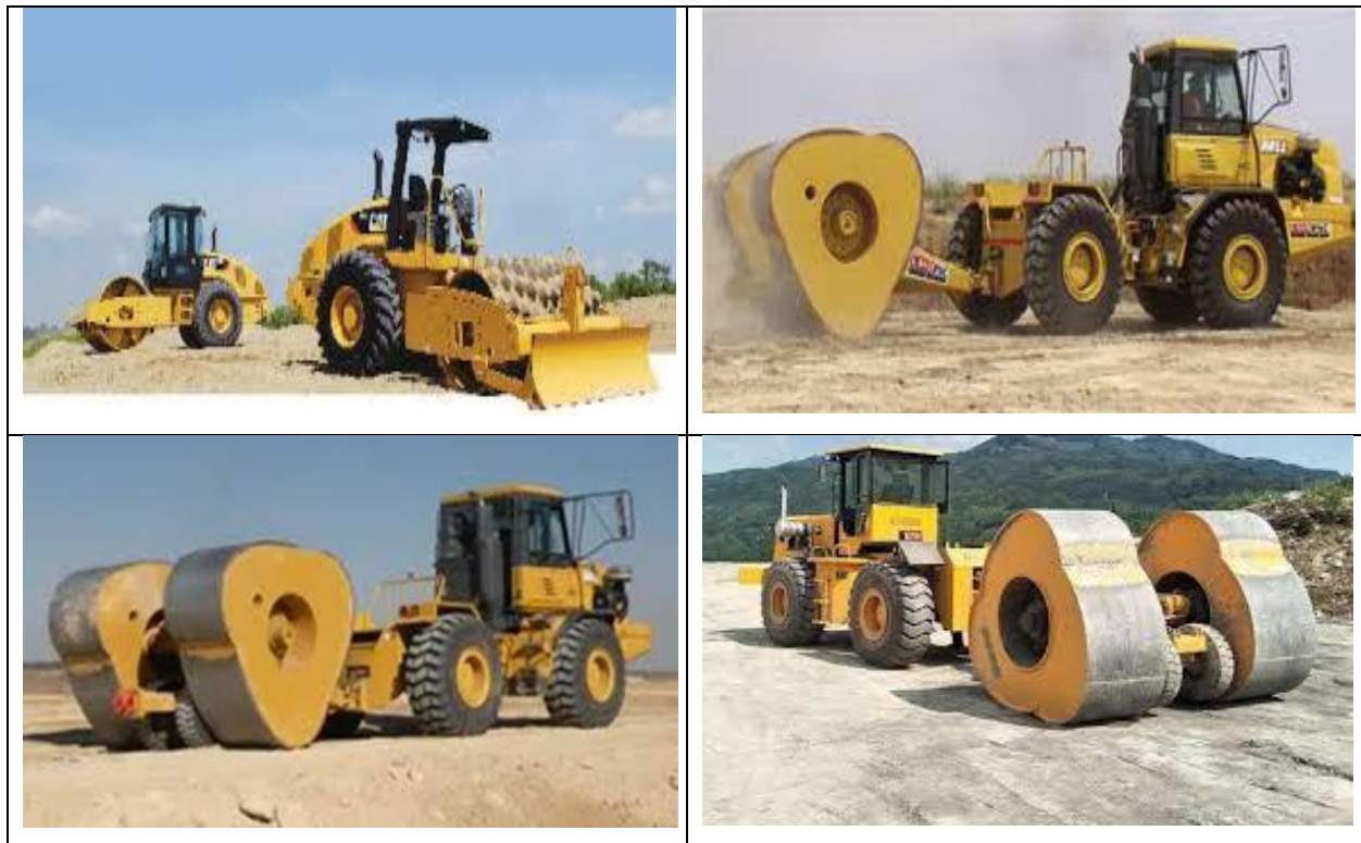
Figure 2.8-Three-Sided Impact Rollers (Jaksa et al., 2019)
