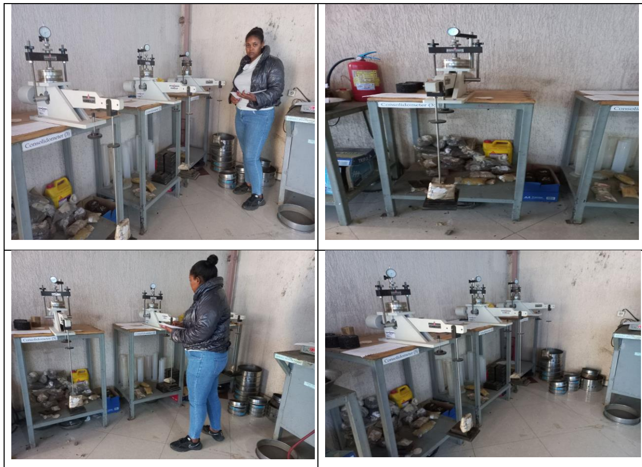
Figure 3-15 Collapse index test
