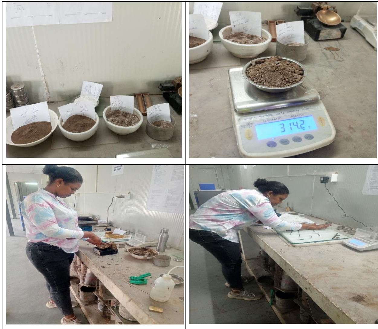
Figure 3-12 Atterberg Limit Test and Sample Preparation
