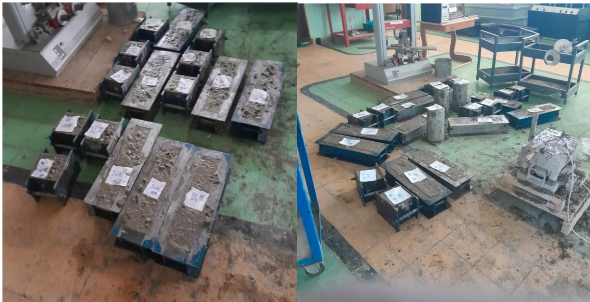
Figure 3.12 Mod preparation and Casting of concrete specimens
