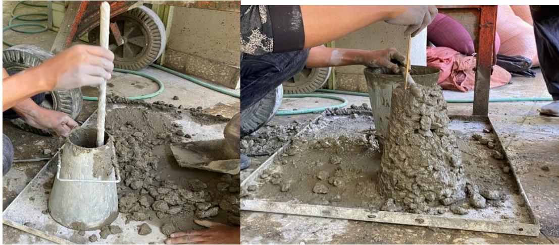
Figure 3.14 Slump taste for concrete mix
