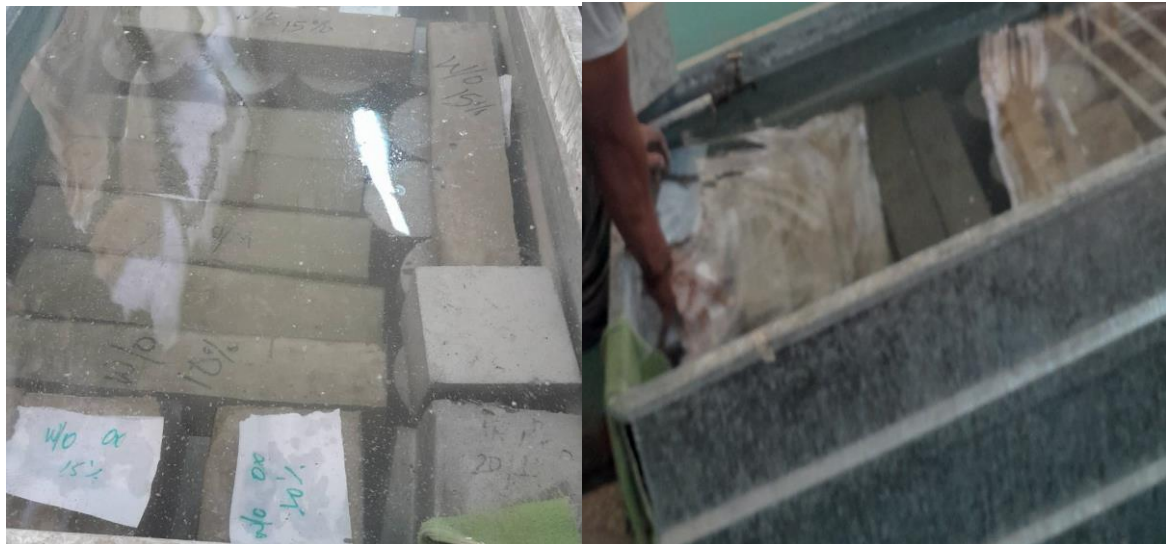
Figure 3.13 curing of concrete specimens and
