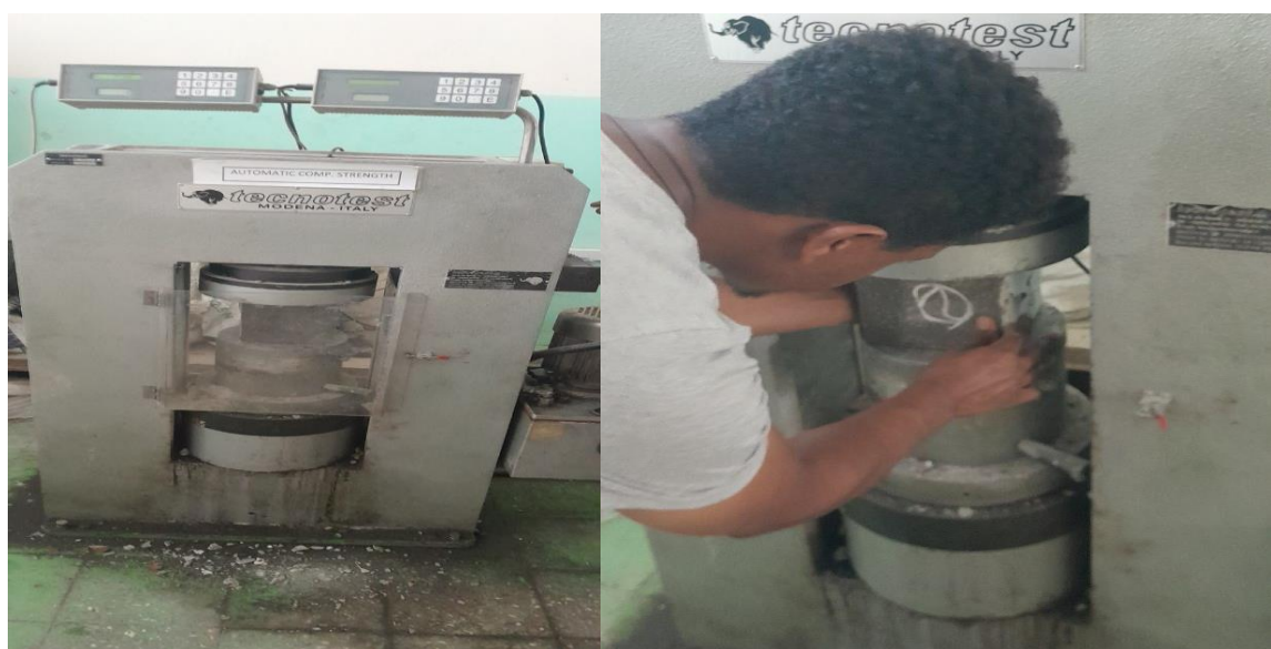
Figure 3.15 Compressive strength taste using Automatic compressive machine.
