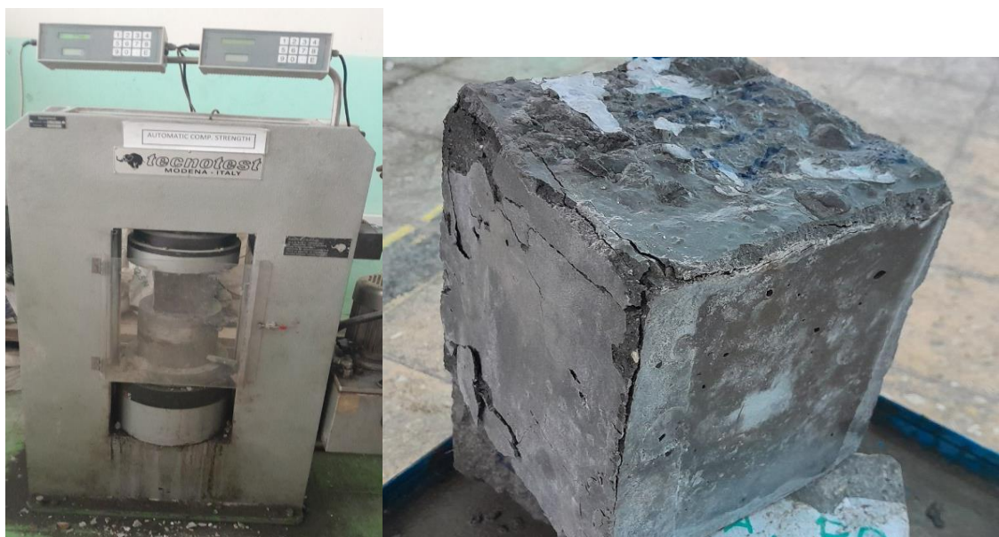
Figure 4.8 a) Compressive test machine b) Cube after compressive strength test
