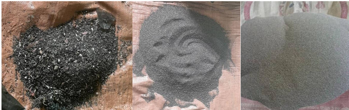
Figure 3.4 Cast iron powder collected and sieved from torno house
