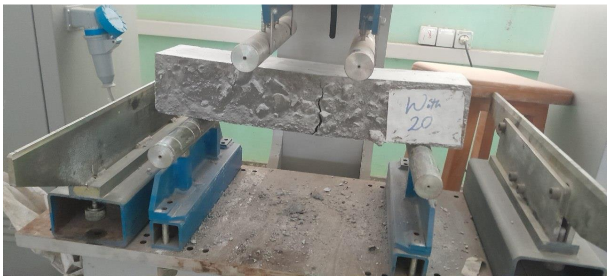
Figure 3.16 Four point loading Flexural Strength testing machine
