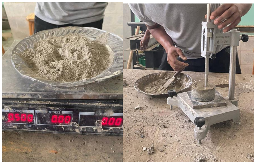
Figure 3.8 Taste for normal consistency of cement paste using vicat apparatus
