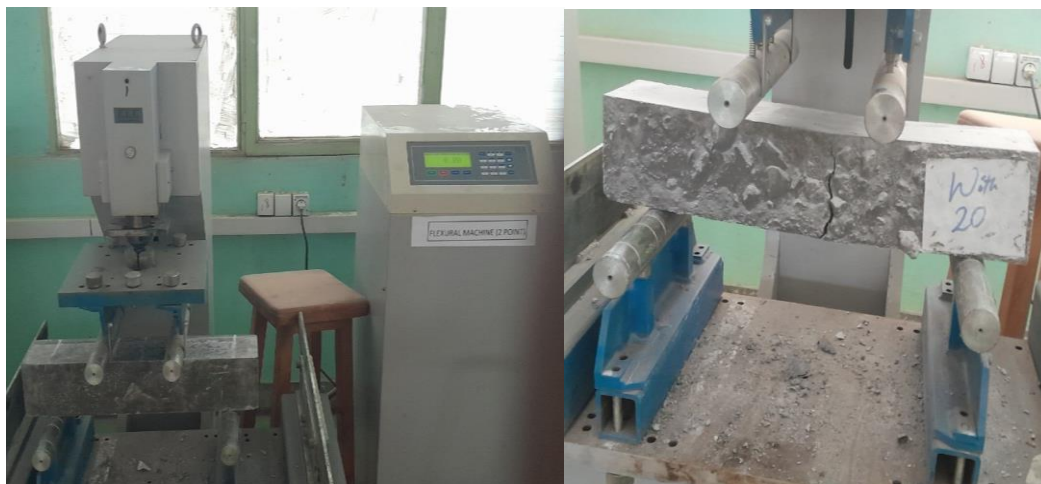
Figure 4.10 The flexural tensile strength tests machine and tested sample
