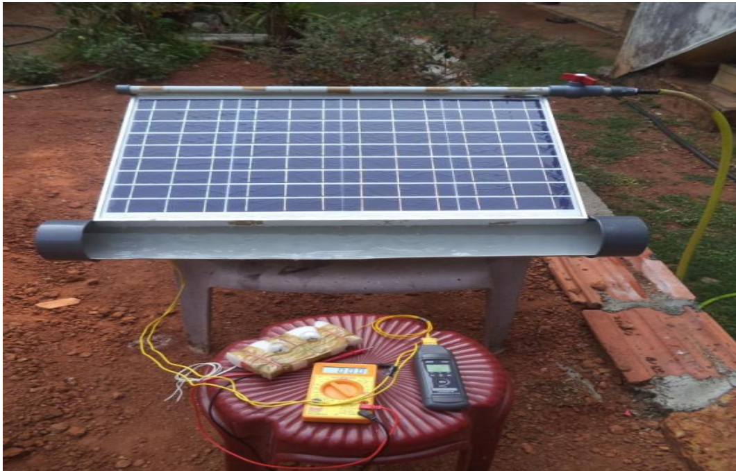
Figure: 2. 5 Photovoltaic modules with free front water flow cooling (Milind et al., 2017)
