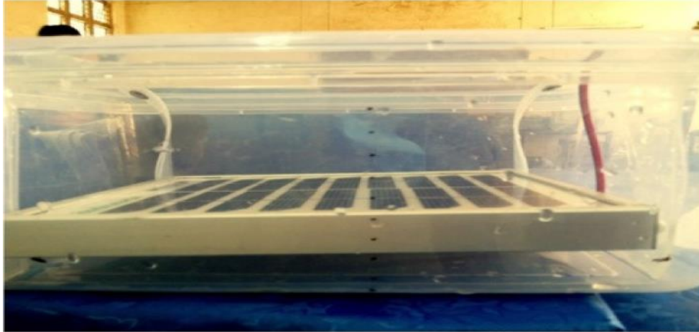
Figure: 2. 6 Photovoltaic immersed in water (Mehrotra et al., 2014)
