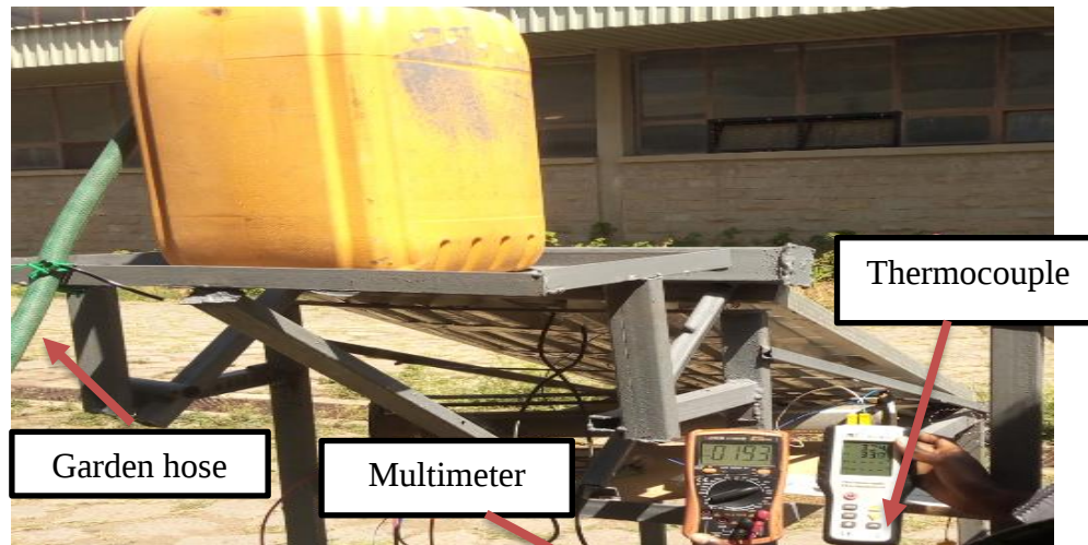
Figure: 4. 6 Voltage and temperature measurement of photovoltaic modules cooled by water
