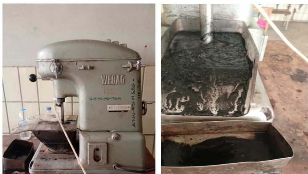
Figure 3-3: Wedag Flotation Machine (left) and flotation process (right)
