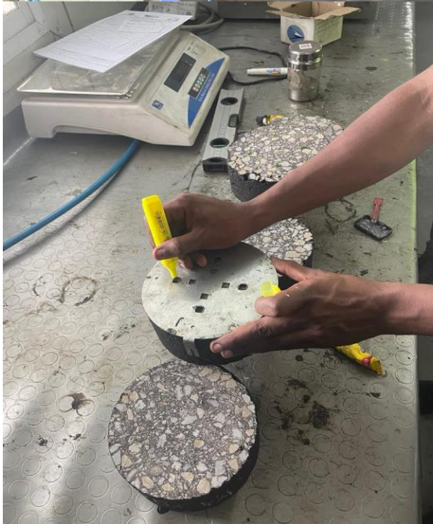
Specimen Preparation for Resilient Modulus, Creep Index and Cracking Tolerance Index Test
