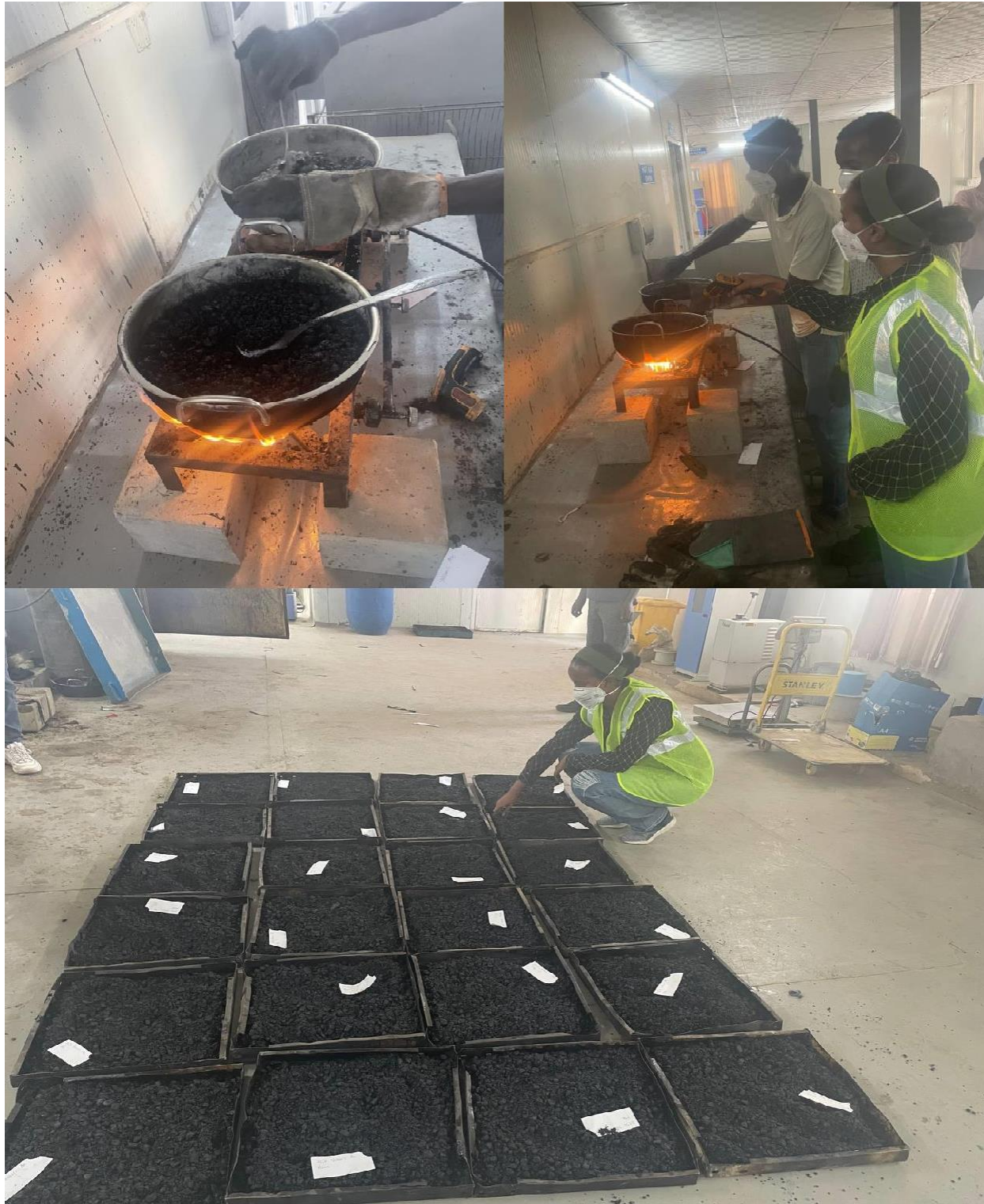
The Preparation Process of Asphalt Mix
