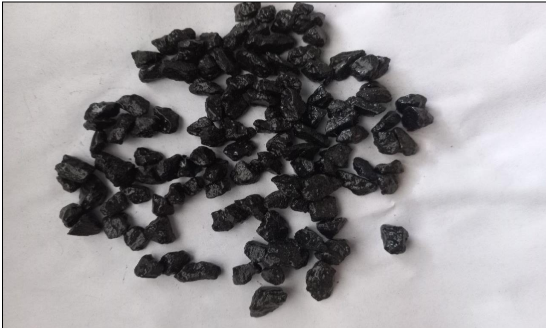
Figure3.3 Aggregates showing over 95% Coating of Bitumen after Static Immersion Test
