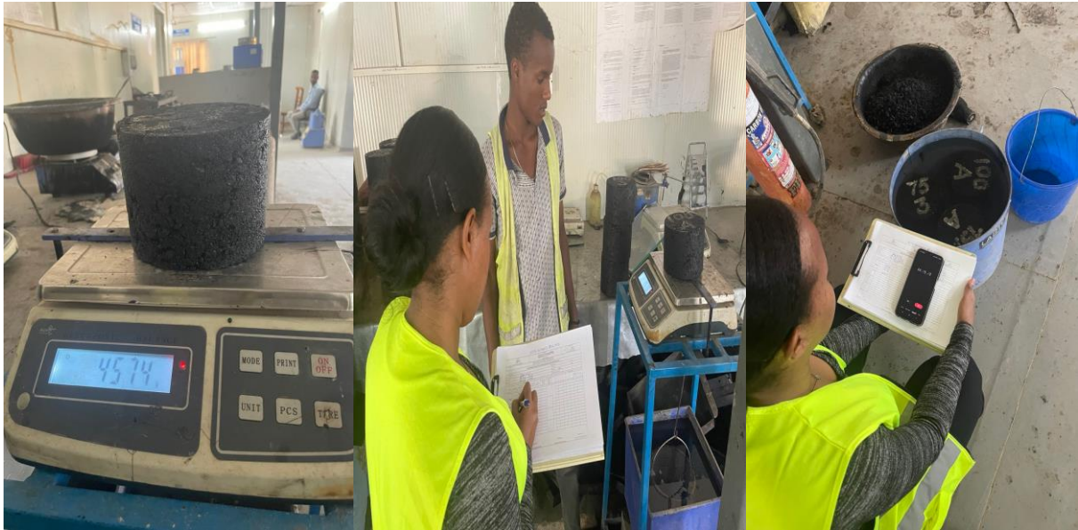
Figure 4.2 Bulk Specific Gravity (Gmb) Testing
