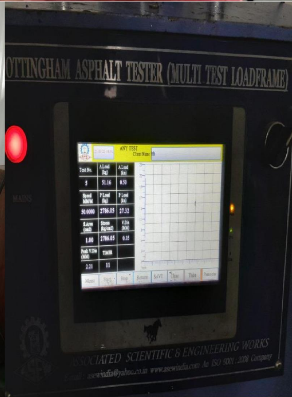
Moisture Susceptibility (Tensile Strength Ratio - TSR) Test
