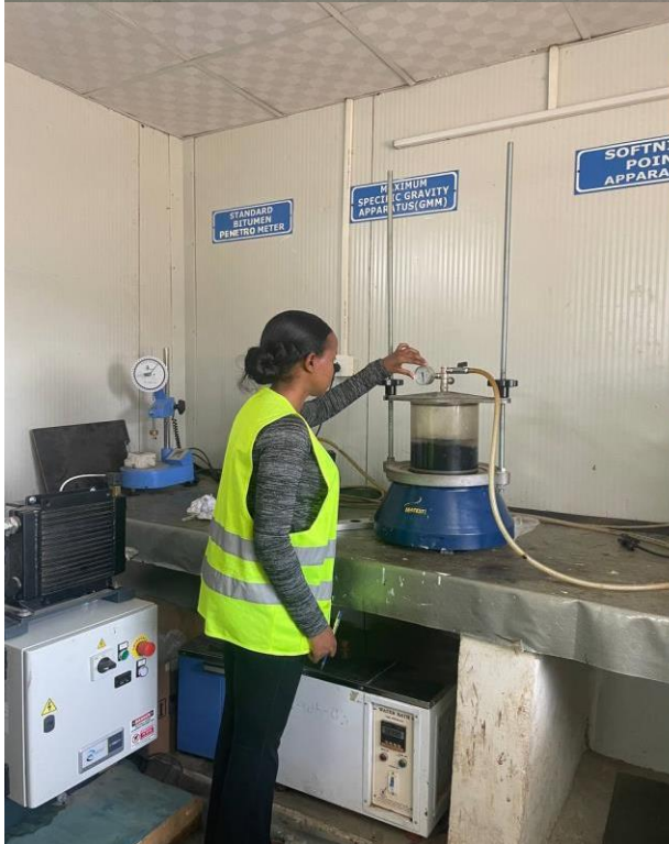
Theoretical Maximum Specific Gravity (Gmm) Test
