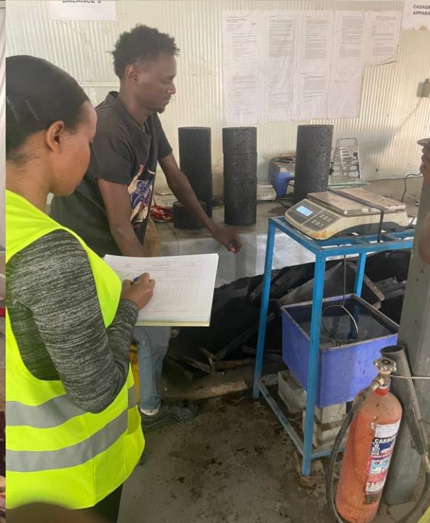
Bulk Specific Gravity Test (Gmb)
