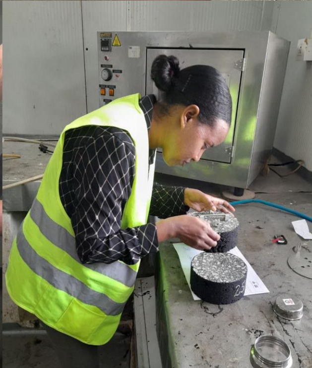
Specimen Preparation for Resilient Modulus, Creep Index and Cracking Tolerance Index Test
