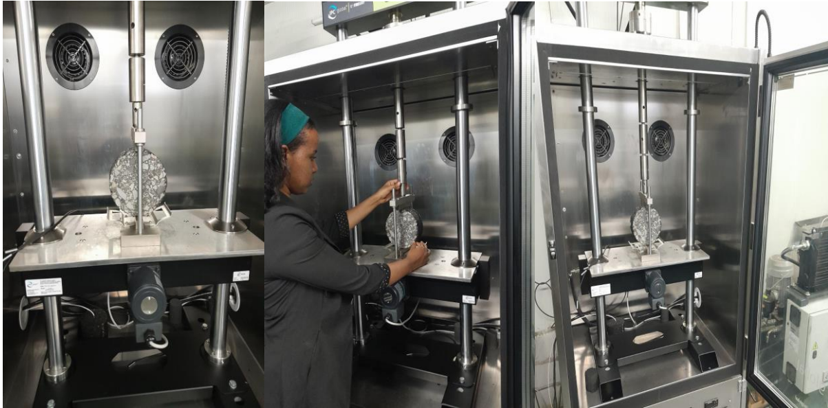
Figure 4.9 Cracking Tolerance Index (CTIndex) Testing
