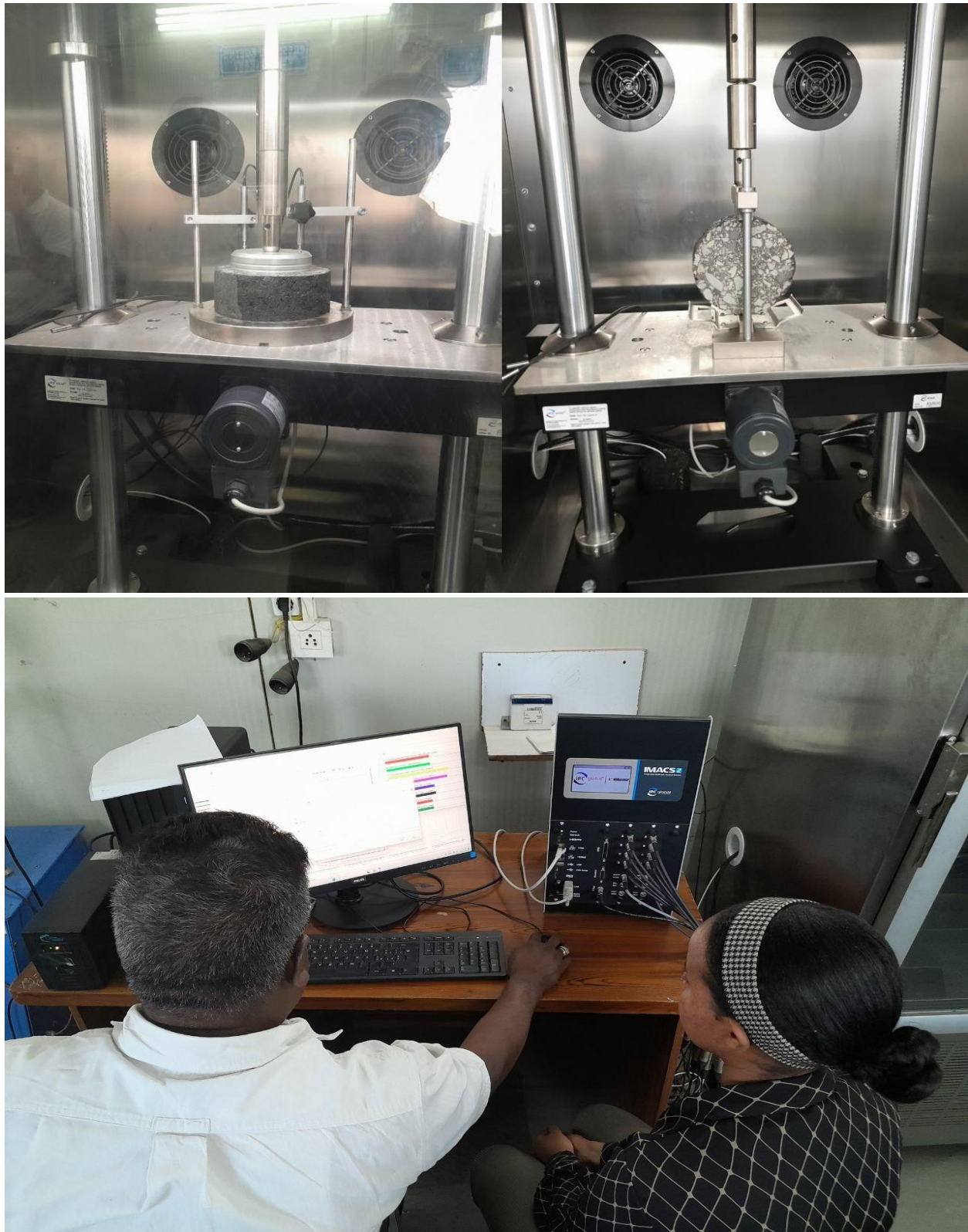
Creep Index and Cracking Tolerance Index Test
