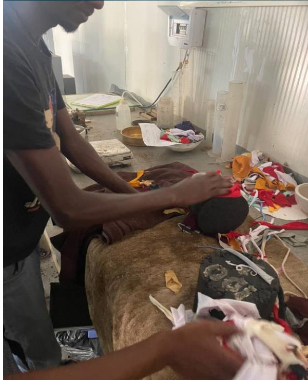
Bulk Specific Gravity Test (Gmb)
