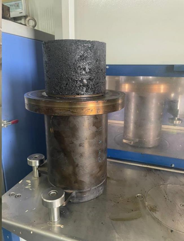
Gyratory Compaction of Asphalt Mix
