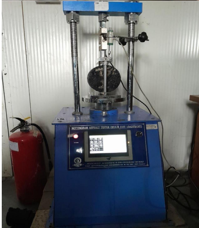
Moisture Susceptibility (Tensile Strength Ratio - TSR) Test
