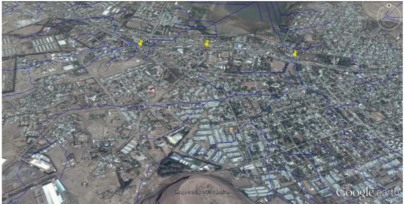
FIGURE 4 2: Drainage Lines from DEM with Satellite Imagery
