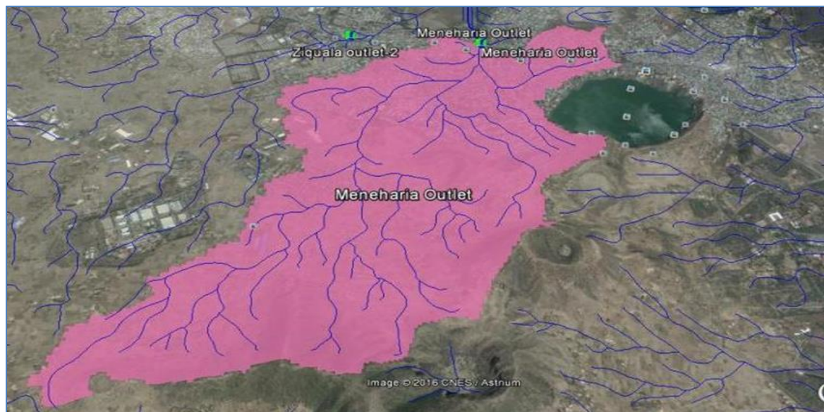
FIGURE 4 10: Meneharia Outlet Catchment & Drainage Lines generated from DEM. Source Drainage Lines generated from DEM with GIS.
