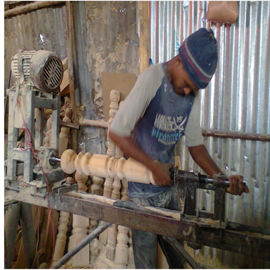
Figure 2.4 locally manufactured wood lathe machine
