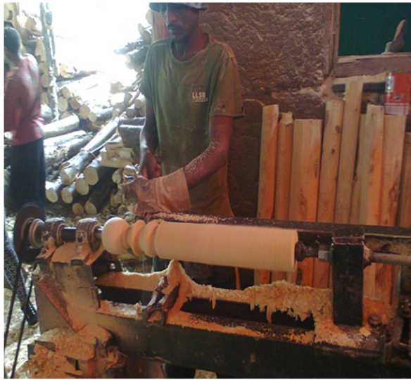
Figure 2.4 locally manufactured wood lathe machine
