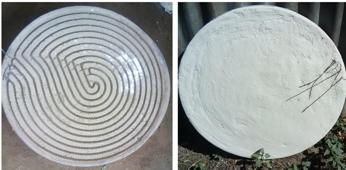
a) Grooving and Embedding Nicrome wire b) Insulating with Gypsum
