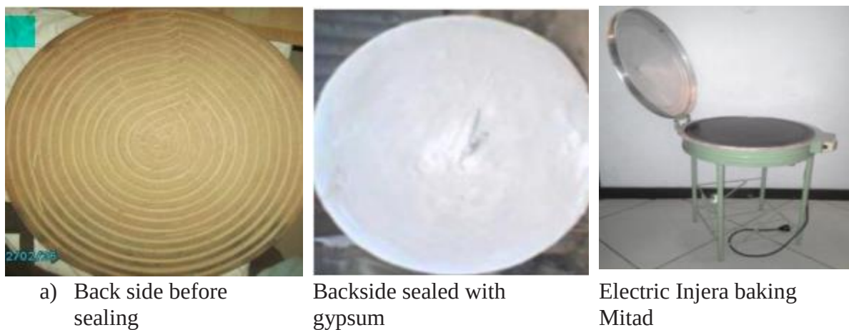
Figure 2.6 Conventional Electric Injera Baking Mitad [7]
