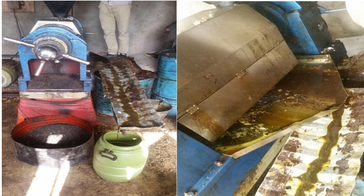
Figure 3-2 Mechanical extraction of argemone Mexicana oil
