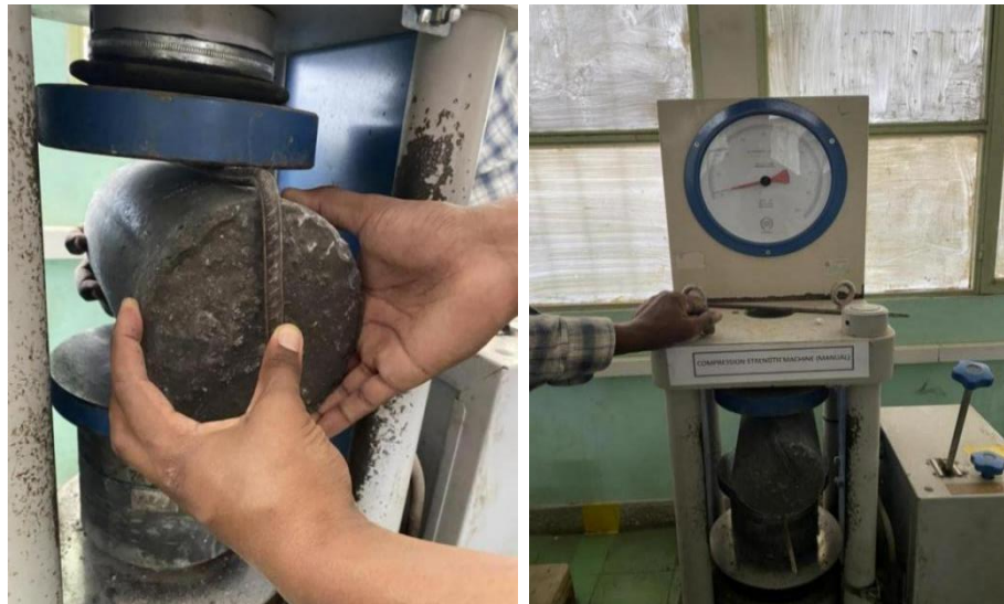
Figure 3.20 Sample mix cast in splitting tensile strength test machine
