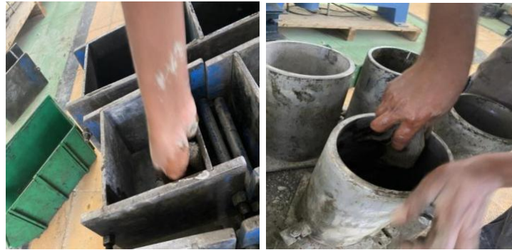
Figure 3.14 Cleaning and lubricating molds
