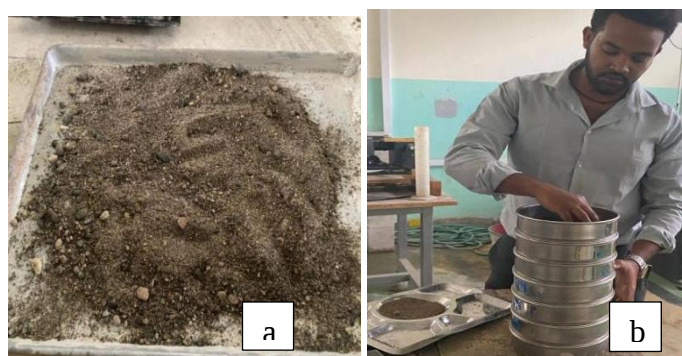
Figure 3.6 Sieve analysis test a) ready sand to be sieved b) sieve analysis test.
