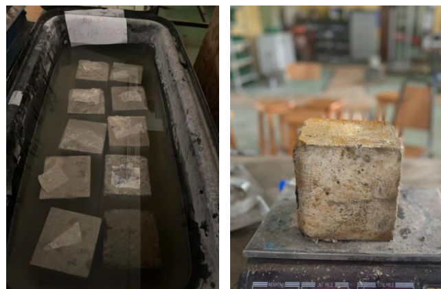
Figure 3.24 Cubes during and after immersed in sodium sulfate solution.
