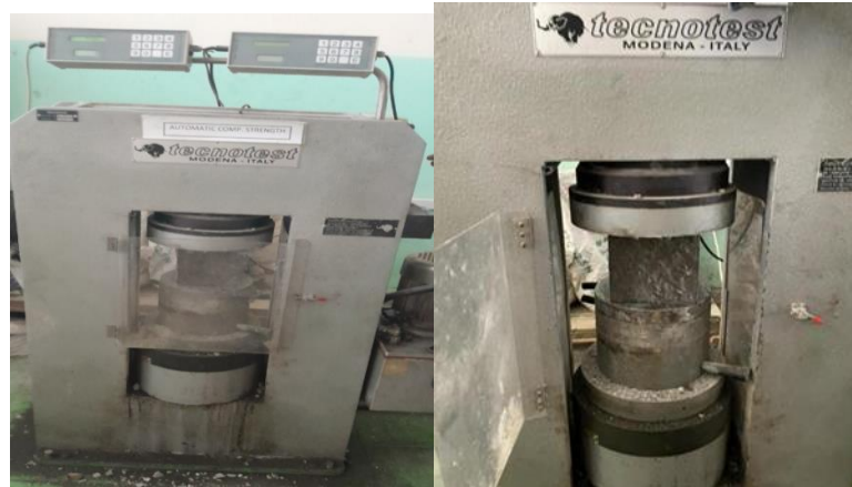
Figure 3.3 Sample mix cube in compressive testing machine
