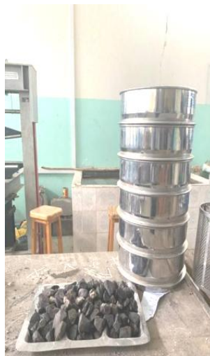
Figure 3.11 Sieve analysis test for coarse aggregate
