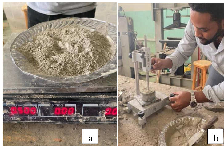
Figure 3.3 Normal consistency tests for OPC a) Cement measurement
