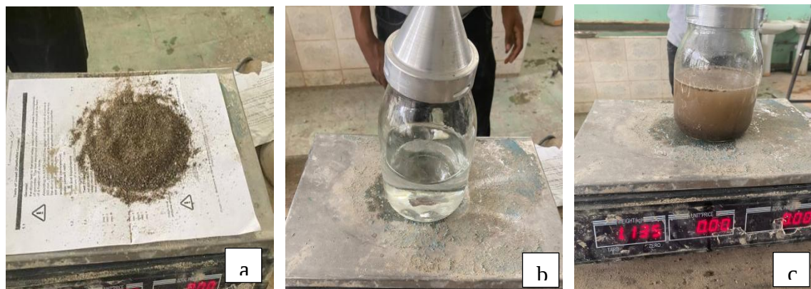
Figure 3.8 Specific gravity and absorption capacity test for fine aggregate a) mass of the sample sand; b) mass of container and water; c) mass of container, water and sand
