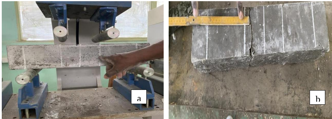
Figure 3.4 Flexural strength test a) Beam ready for flexural test b) Beam after flexural test (rupture inside middle third)
