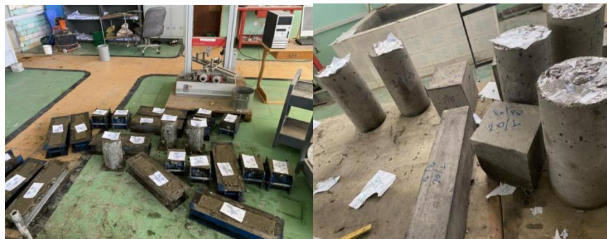
Figure 3.17 Sample concrete specimens before and after casting for 24hrs.
