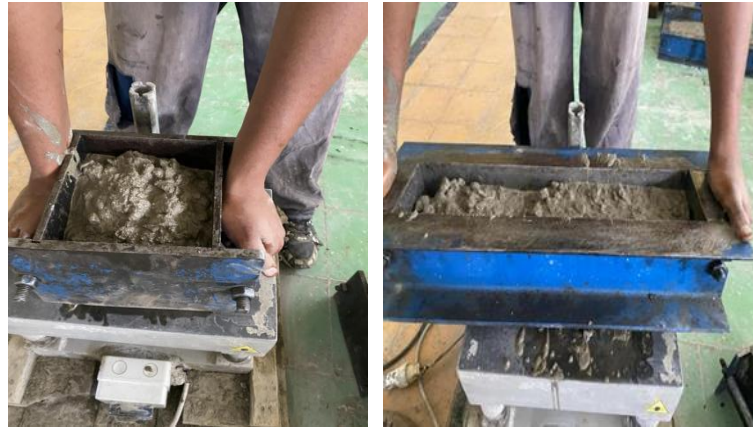
Figure 3.16 Compacting molds using vibrating table compactor
