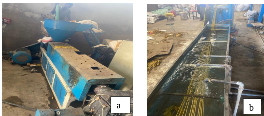
Figure D-2 Melting and Extrusion a) Melting b) Extrusion and solidification through water
