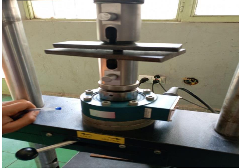
Figure 3-6 Universal testing machine (UTM) setup for compression test
