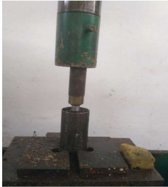
Figure 3-12 Hot extrusion setup
