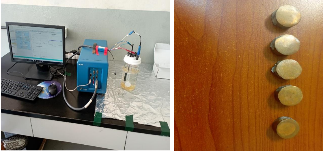
Figure 3-7 Corrosion test set up (a) potentiator setup for corrosion test and (b) sample prepared for corrosion test
