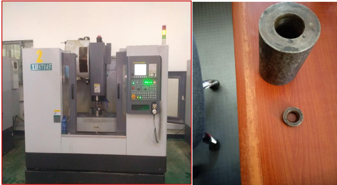
Figure 3-11 Die fabrication setup and fabricated die
