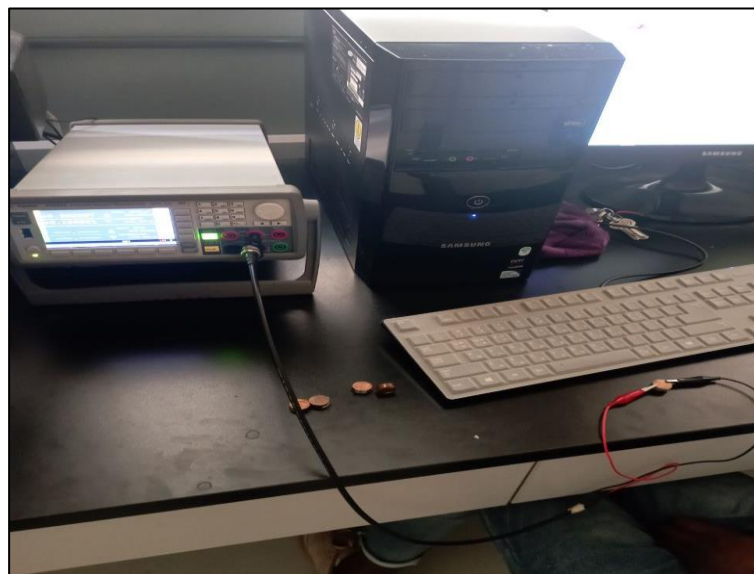
Figure 3-8 Precision source measuring unit set up for electrical conductivity test
