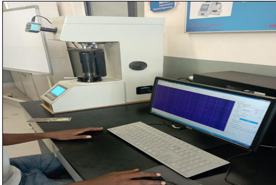
Figure 3-5 Vickers hardness testing machine set up
