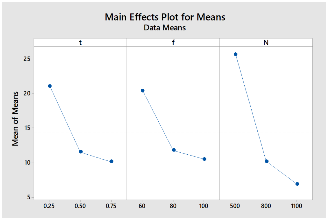
Figure 4.26 Main Effects Plot for Means of Tool Life for Wet Turning
