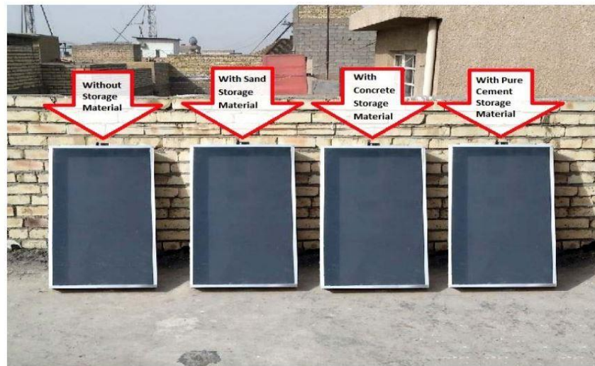
Figure 2.6: Flat plate solar air heater with different sensible thermal storage material (Saravanakumar and Mayilsamy, 2010)
