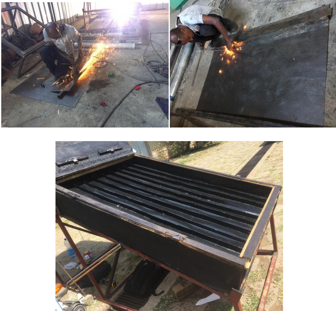
Figure 3.15: Collector absorber plate construction
