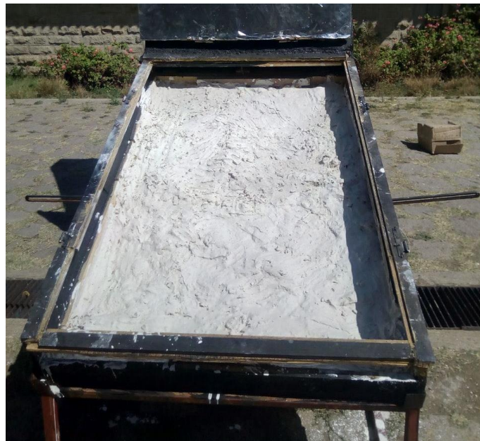
Figure 3.17: Preparation of gypsum into bottom of absorber
