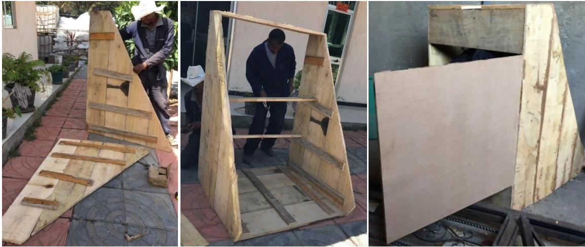
Figure 3.20: Dryer box Construction
