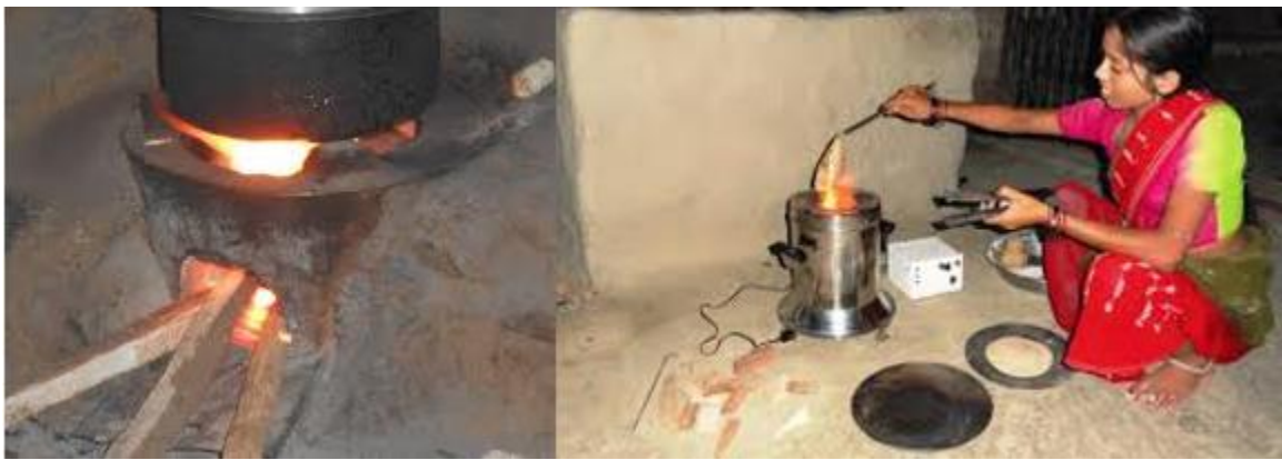
Figure 2.4 Natural and forced draft improved biomass cookstoves (Kar et al. , 2012)
