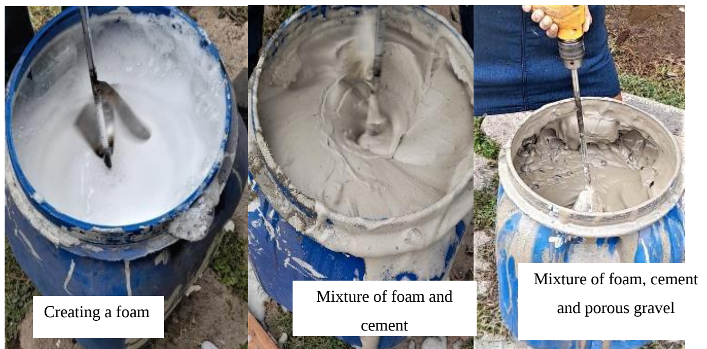
Figure 5.1 Preparation of Aircrete mixture
