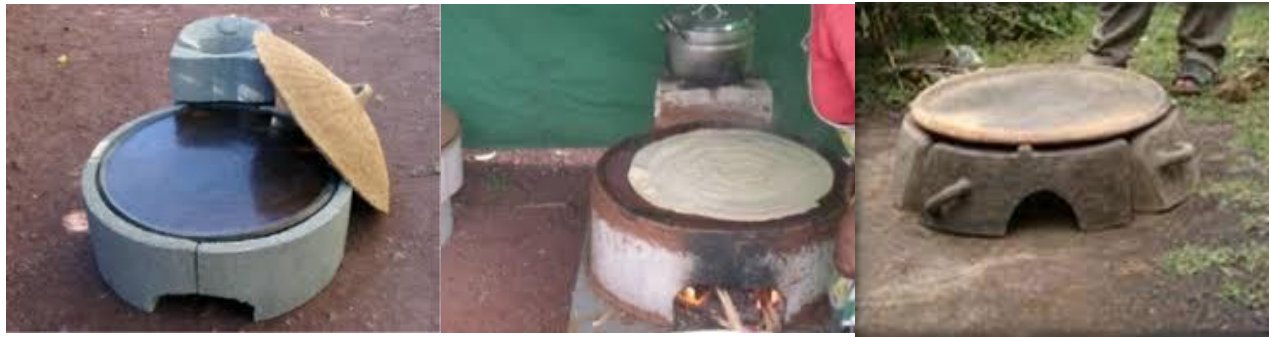
Figure 2.3 Improved biomass cookstove (Amare et al. , 2015)
