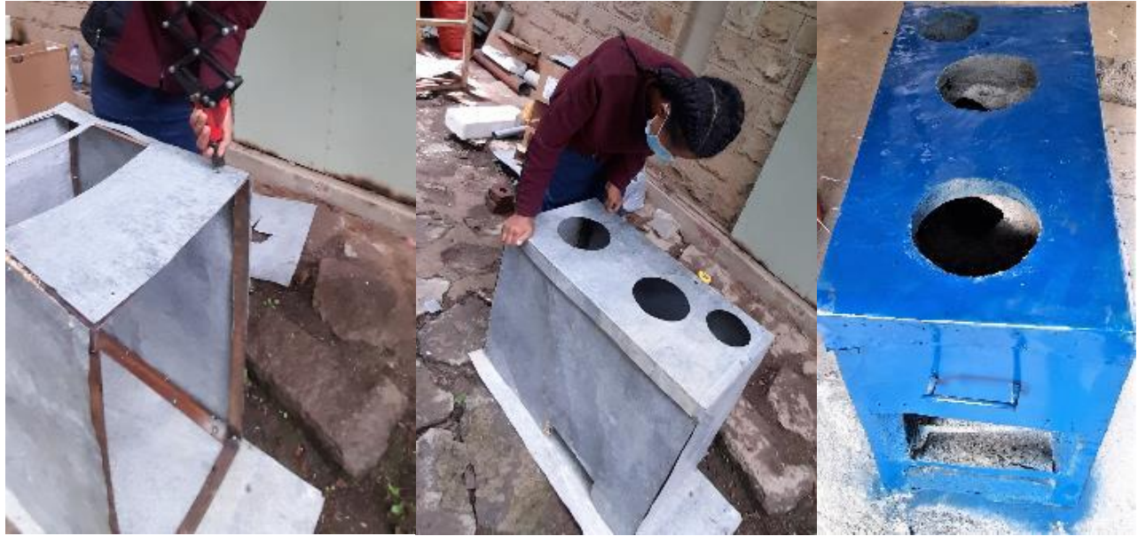
Figure 5.11 Assemblies and mold of the stove
