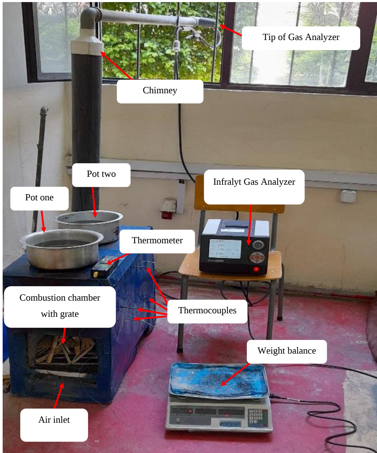
Figure 5.12 Experimental setups of double-pot biomass stove
