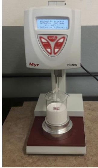
Figure 3. 3. Viscosity measurement of traffic marking paint.
