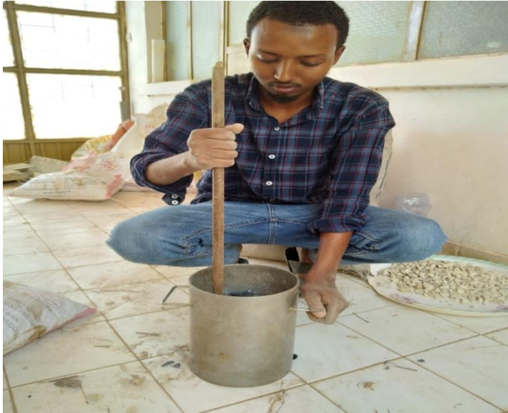
Figure 5 Aggregates filled in container by striking with 25 strokes
