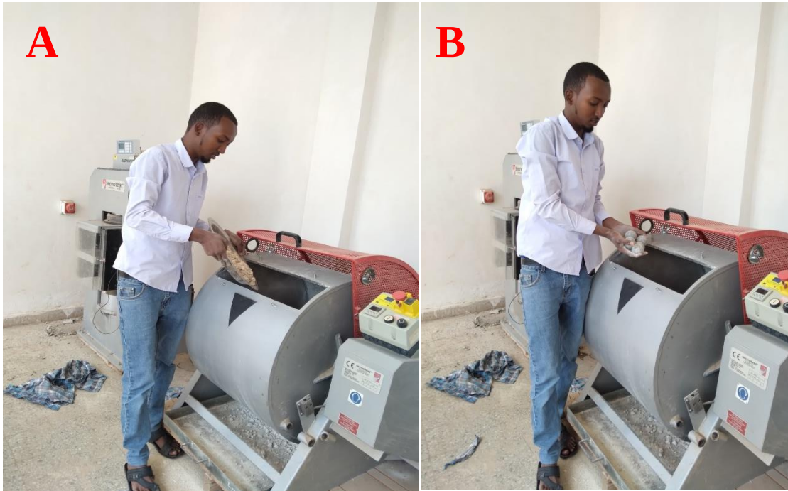
Figure 9 Aggregates loaded in abrasion machine (A) steel balls charged together with aggregates (B)
