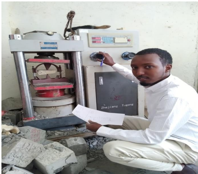
Figure 3 Pont load test
