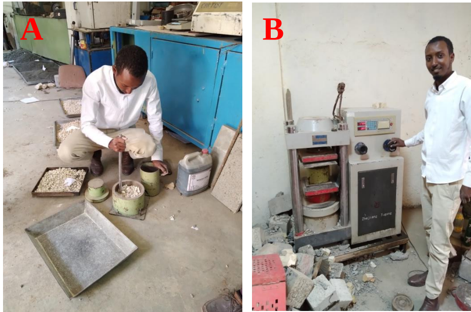
Figure 7 Aggregates filled in cylindrical steel cup (A) aggregate placed in compression machine
