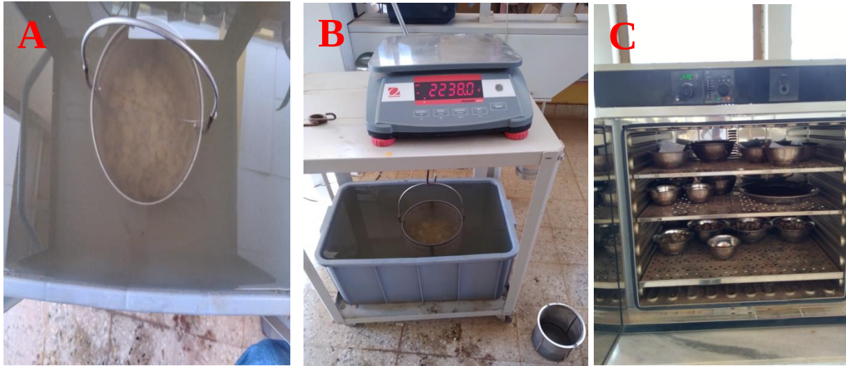
Figure 6 Aggregates soaked in water (A) Apparent mass (B) and Aggregates in oven(C)
