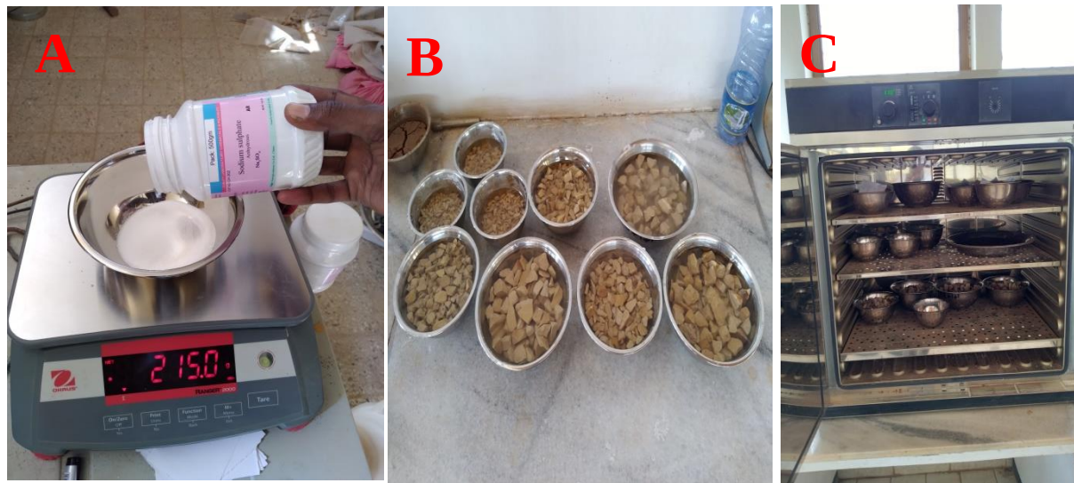
Figure 10 Sodium sulphate powder (A) Aggregate immersed in sodium sulphate solution (B) Aggregate placed in oven (C)
