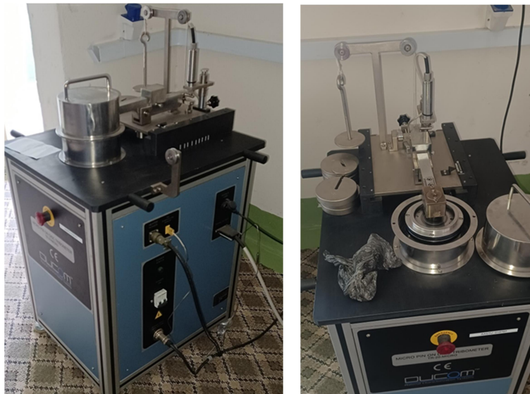
Figure 9: photograph image of real manufactured PIN on DISC wear test machine
