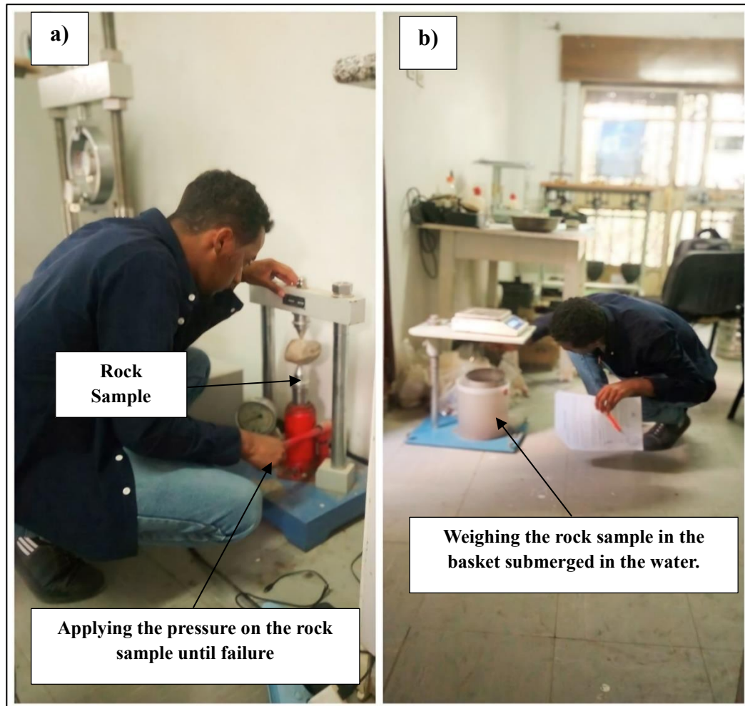
Figure 3. 3. Rock sample analysis in the laboratory. a) point load index test, and b) water absorption determination.
