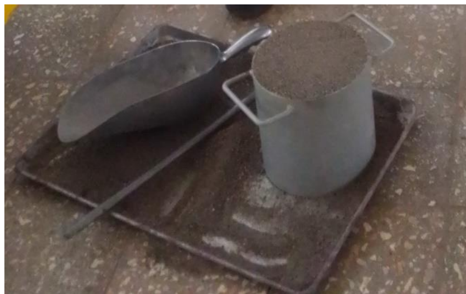
Figure 3.5 Unit weight measurement of fine aggregate
