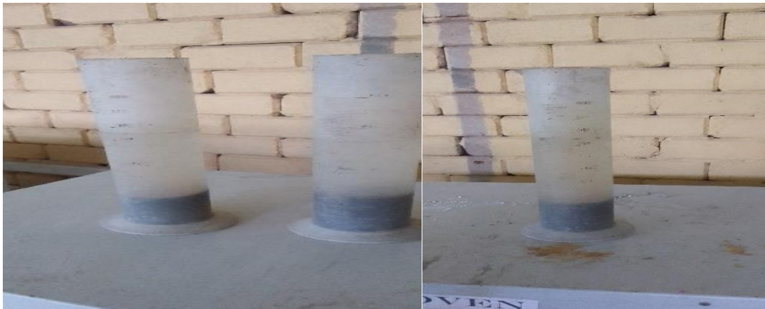
Figure 3.4 Silt content test
