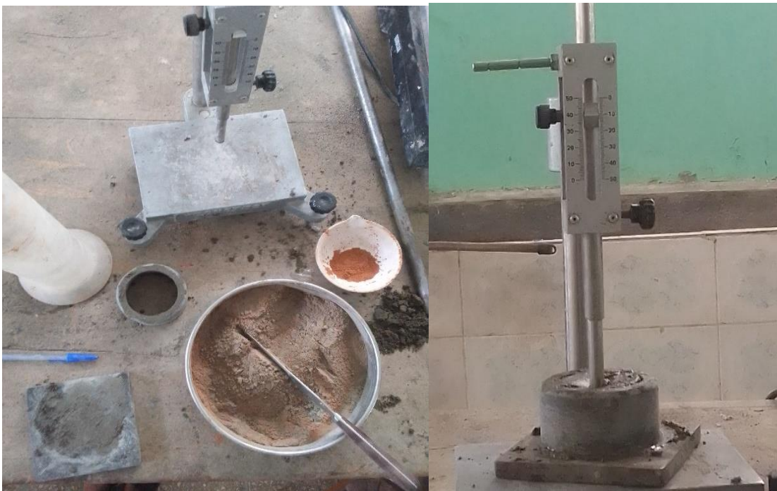
Appendix E2: Picture taken during normal consistency and setting time test.
