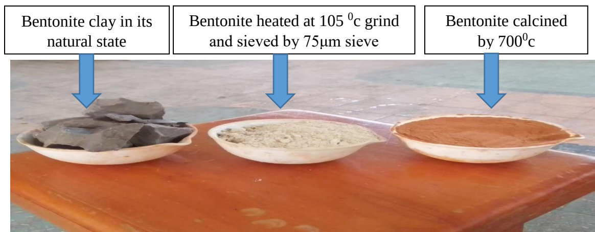
Figure 4.4 Bentonite preparation process
