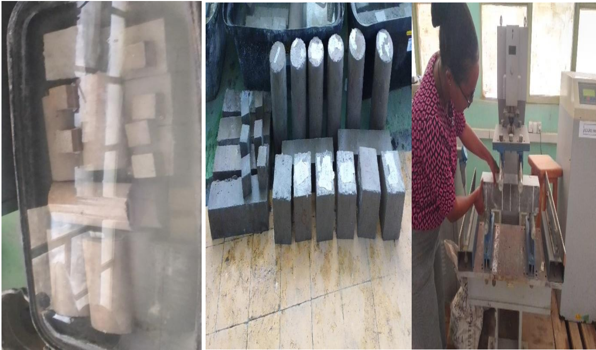
Appendix E5: Pictures captured during curing, surface drying and testing of concrete.
