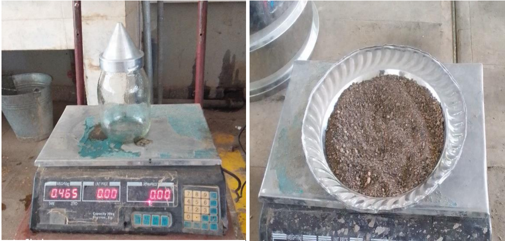
Figure 3.6 Specific gravity and water absorption of fine aggregate
