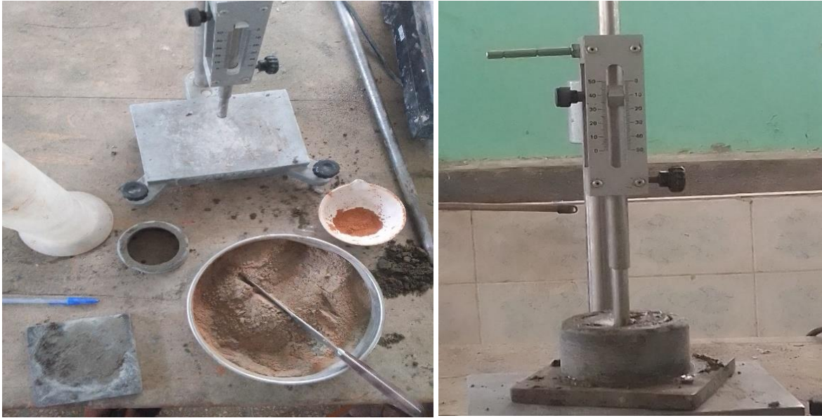
Figure 3.9 Normal consistency test for cement
