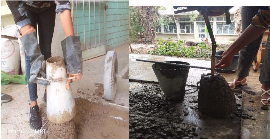
Figure 4.10 Workability test of concrete by slump cone
