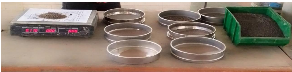
Figure 4.1 Sieve analysis test of fine aggregate
