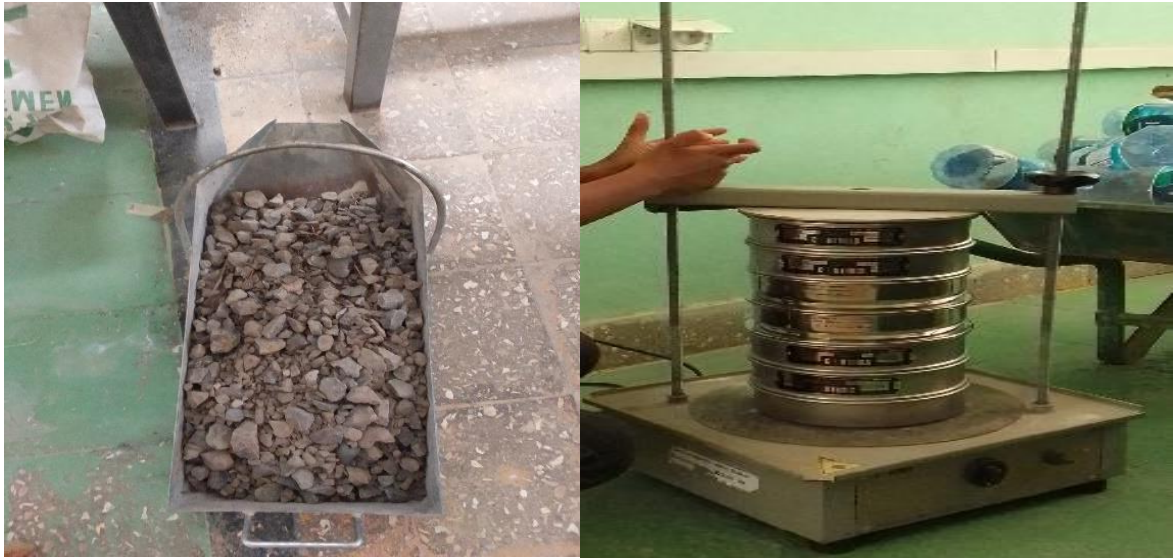
Figure 3.7 Sieve analysis of coarse aggregate
