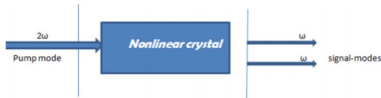
Fig. 2.3: A degenerate parametric amplifier with nonlinear crystal pumped by coherent light (Getahun, 2019).
