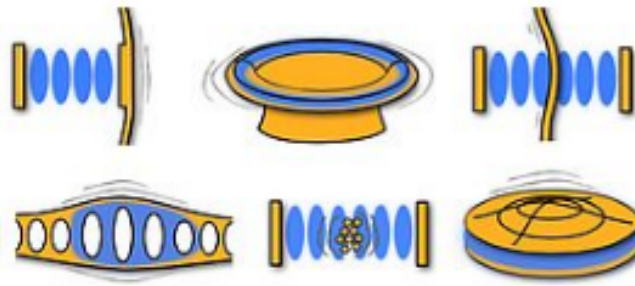
Fig. 2.1: Optomechanical Setups (schematic), from top left: Fabry-Perot cavity with a moveable end-mirror, microtoroid, membrane or nanotube inside a cavity, photonic crystal, atoms trapped inside a cavity, vibrating capacitor plates in a microwave LC circuit (Marquardt and Girvin, 2009).
