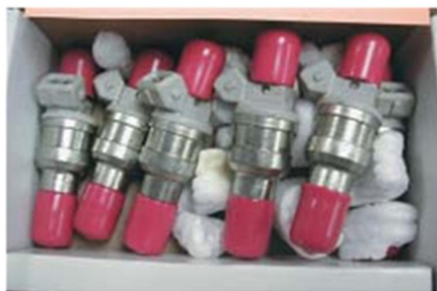
Figure 25: A standard electrical solenoid injector new
