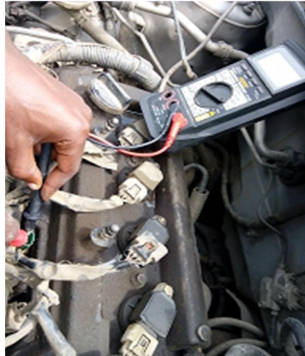
Figure 29: measure the resistance of injectors
