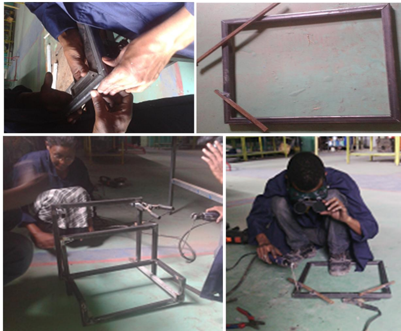
Figure 37: the group members at work in the making of the frame structure
