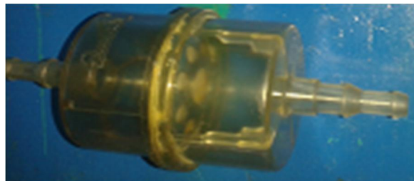
Figure 42: fuel filter used for the developed tester
