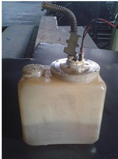
Figure 40: plastic fuel tank and fuel pump used for the tester fabrication
