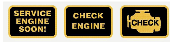
Figure 17: Malfunctioning indicator light
