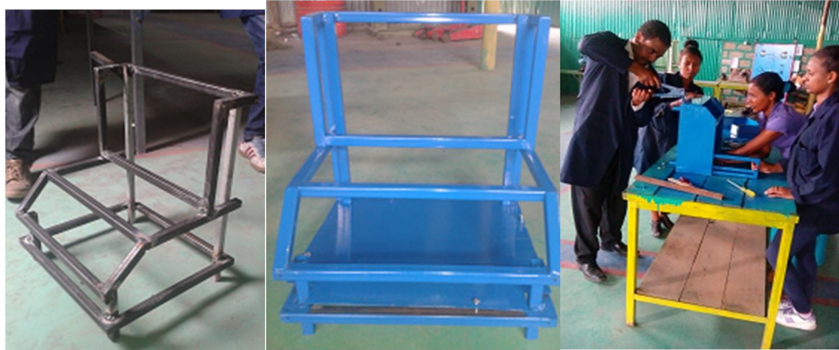
Figure 38: the group member at work in finalizing the making of the frame structure
