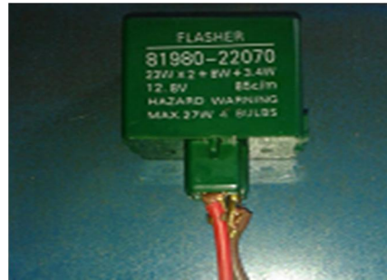
Figure 52: Flasher used in the tester
