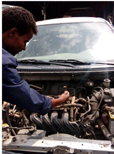
Figure 30: disconnecting electrical connections to remove from the injector
