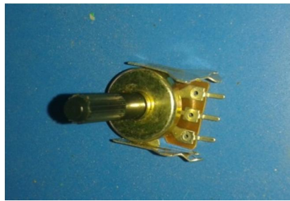
Figure 54: variable resistor used in the tester
