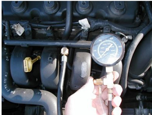
Figure 19: pressure regulator testing
