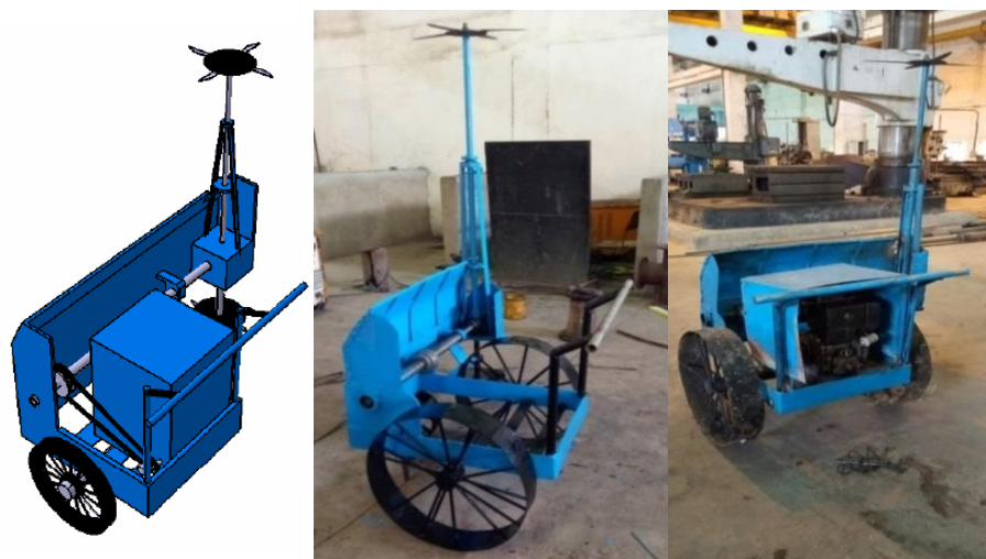
Figure 3. 16. Machine model and construction of machine in the shop
