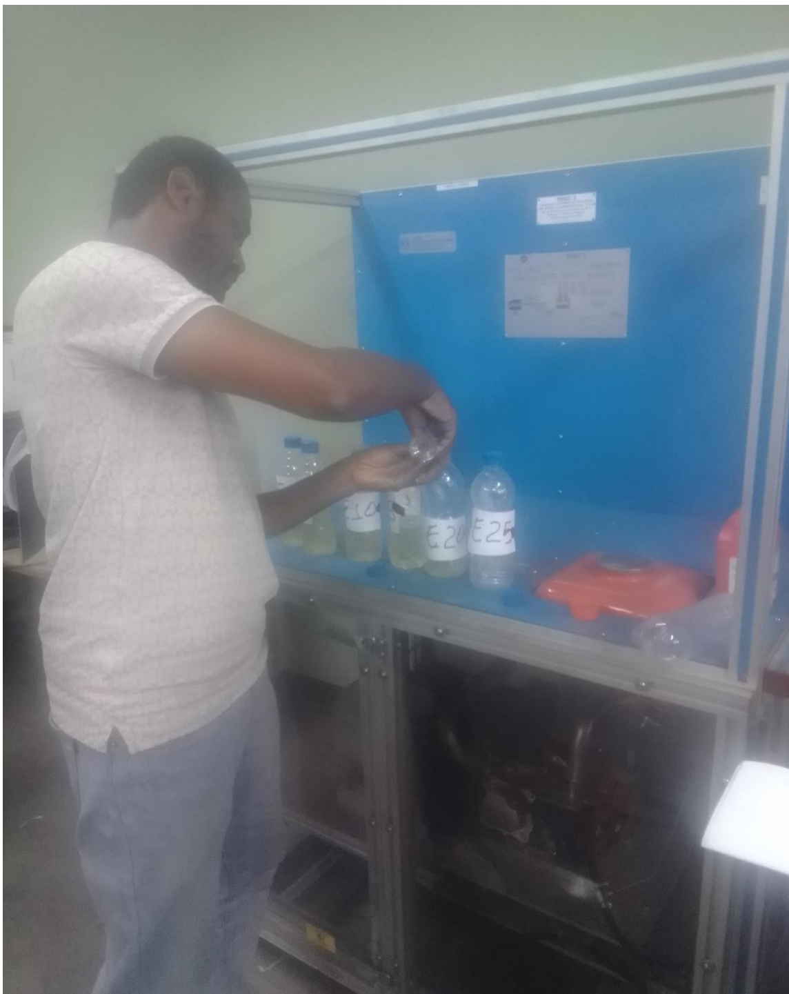
Appendix 4.35 Test fuel blend preparation
