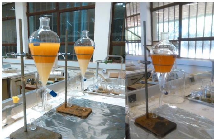
Figure 3.7 First and final (sixth step) biodiesel washing
