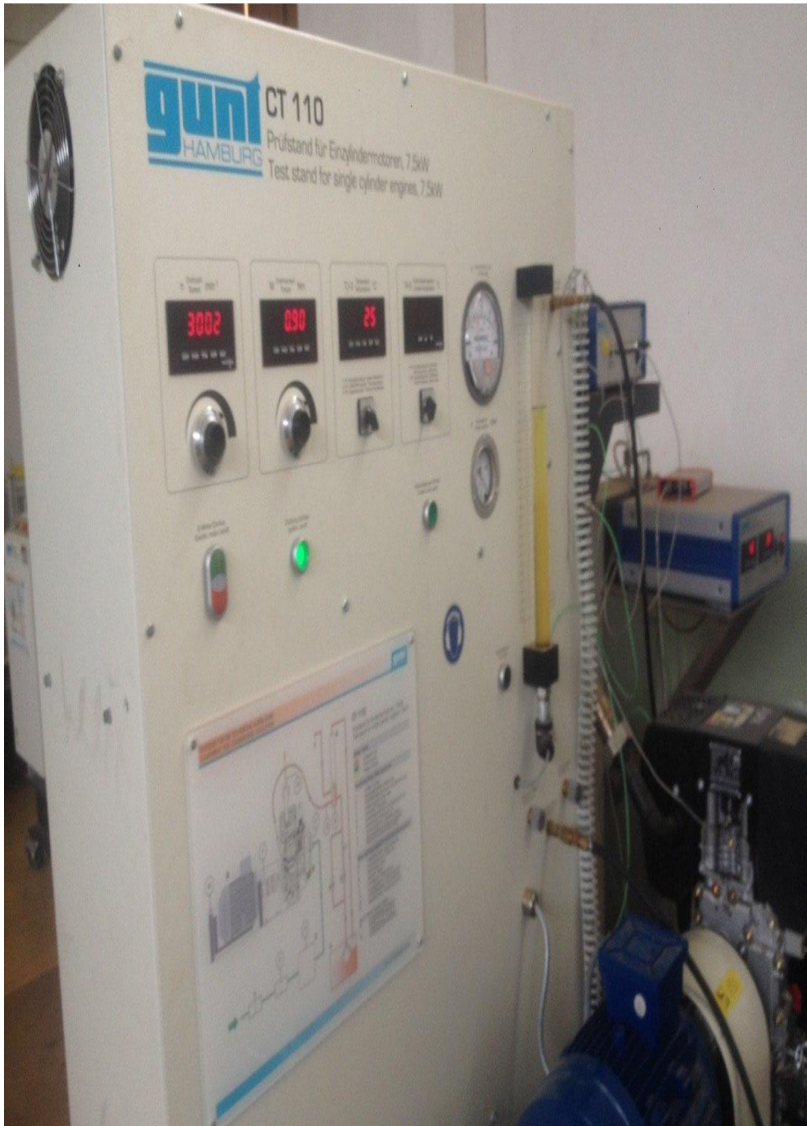
Test stand set at engine speed 3000rpm and full load set near 10
