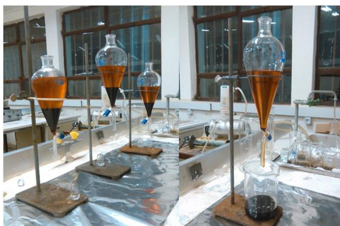
Figure 3.6 Separation of crude biodiesel and glycerin phase
