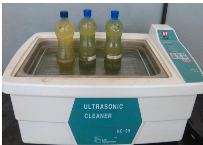
Figure 3.10 Preparation of blended fuels with NPs in Ultrasonicator cleaner.
