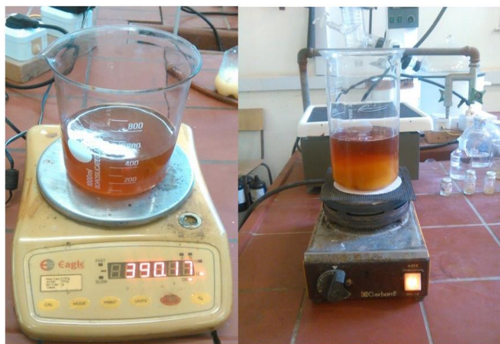
Figure 3.3 Measuring and preheating of UCO before transesterification reaction
