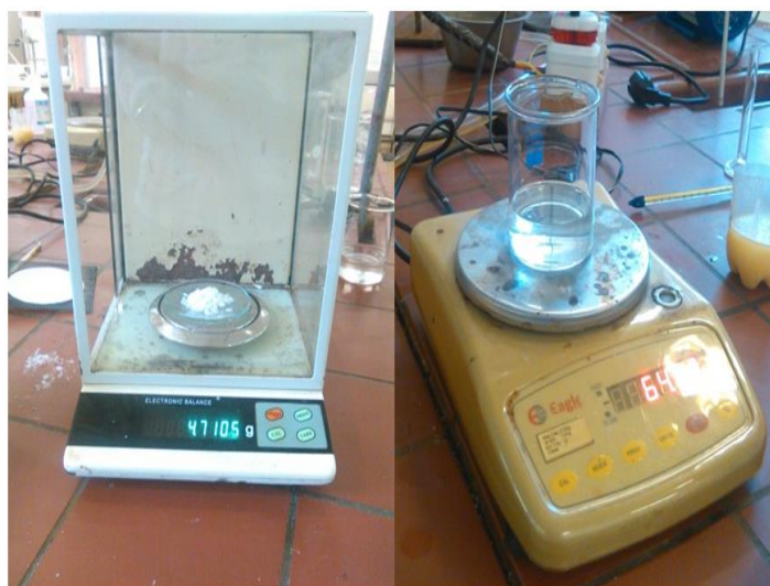
Figure 3.4 Measuring of potassium hydroxide and methanol
