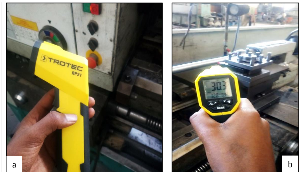
Figure 3.7. TROTEC BP21 Infrared thermometer; a) Side view and b) Front view
