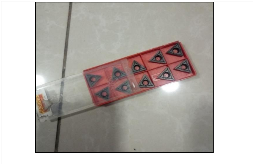
Figure 3.2. Image of carbide cutting tool used (TCMT 16T308)
