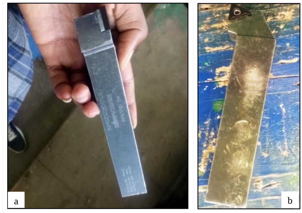
Figure 3.3. STGCR2525M16 tool holder; a) Side view b) Front view
