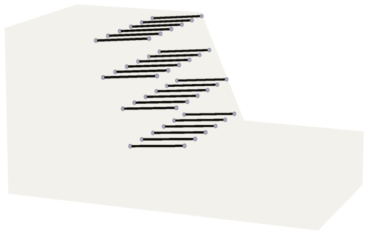
Model developed with nail of 3.5m length, 15 inclination, 1.75m space and 16mm of diameter.
