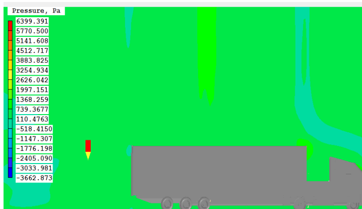
Figure 27: Model 1 velocity and pressure distribution (64km/h)
