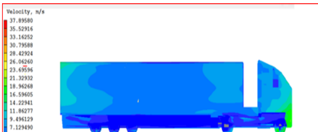
Figure 35: Total Pressure and Velocity contour for simulations at Y= 900mm
