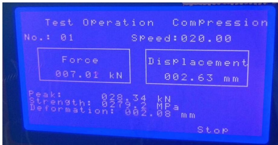
Figure 4.18: A1 compression test for 90^\circ fiber orientation
