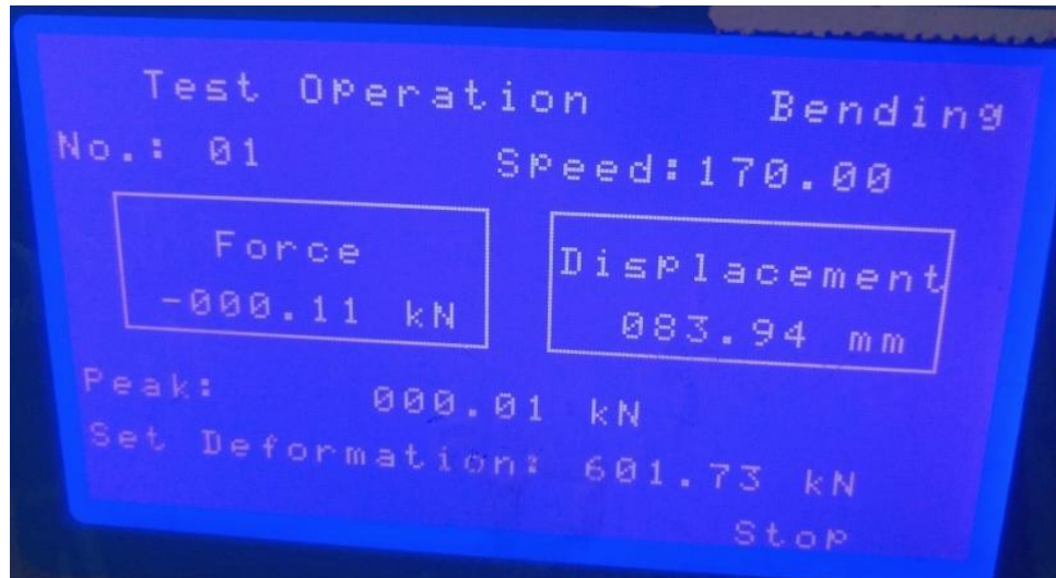
Figure 4.29: A3 0/90 fiber orientation flexural test
