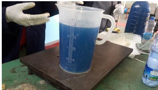
Figure 3.7: Preparation of polyester with hardener.
