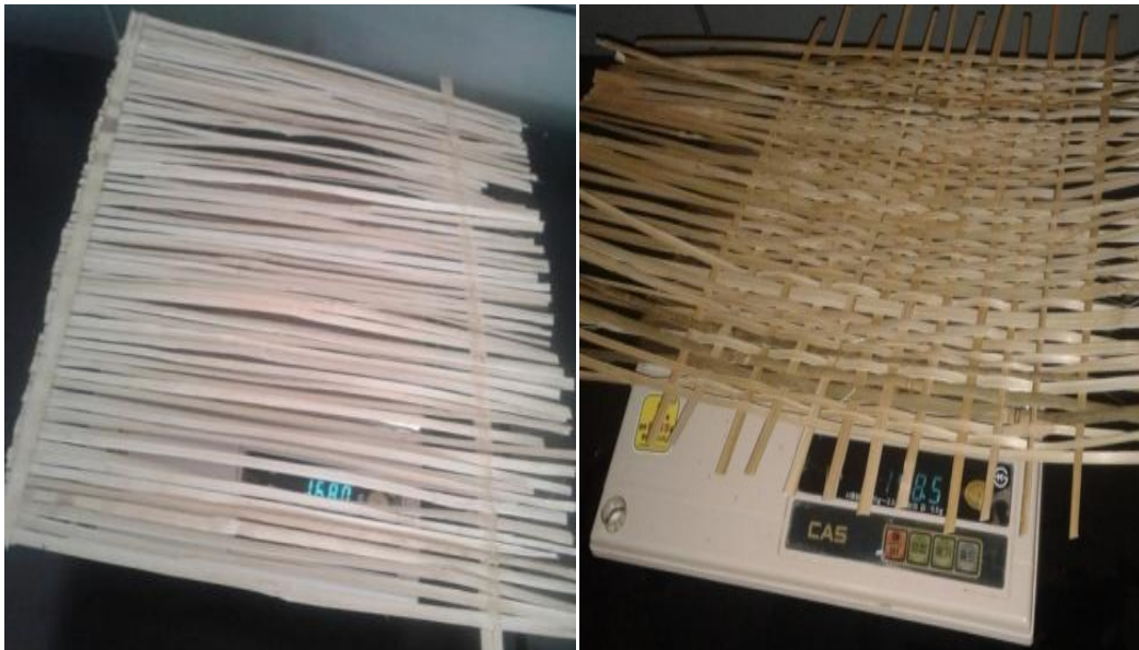
Figure 3.5: measuring weight of unidirectional & woven bamboo fiber
