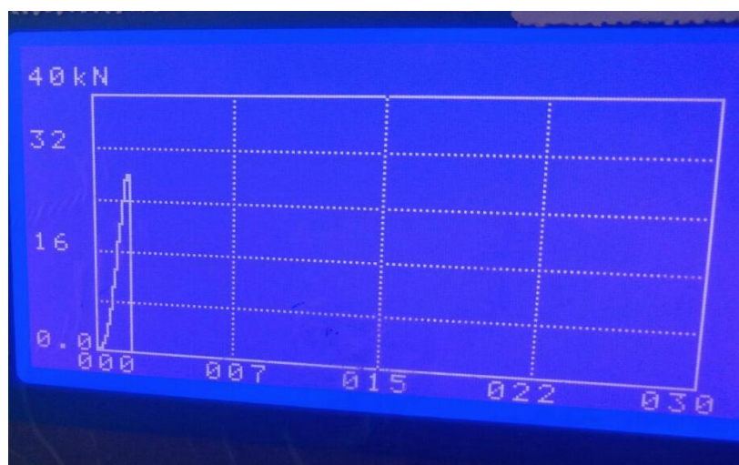
Figure 4.19: 90^\circ fiber composite peak load Vs deformation
