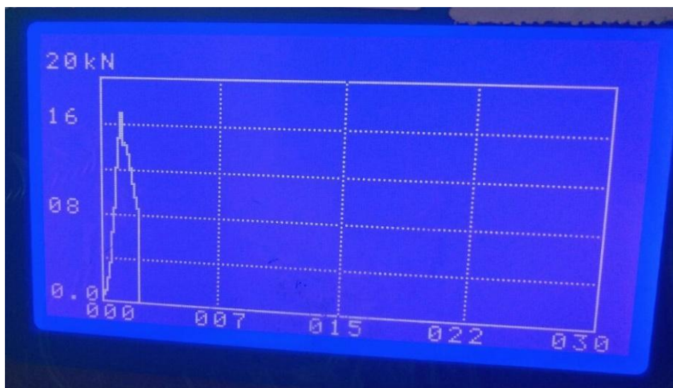
Figure 4.23: 0/90^0 fiber orientation composite peak load (kN) Vs deformation (mm)
