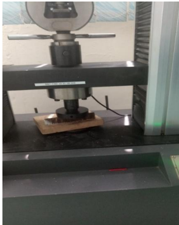
Figure 4.17: Compression test setup
