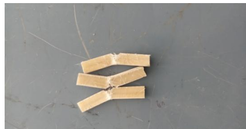
Figure: 4.34 Sample Specimens after impact test
