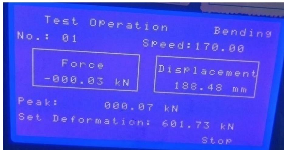
Figure 4.28: A2 0° fiber orientation flexural test
