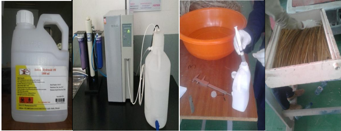
Figure 3.2: Bamboo strips chemical treatment process
