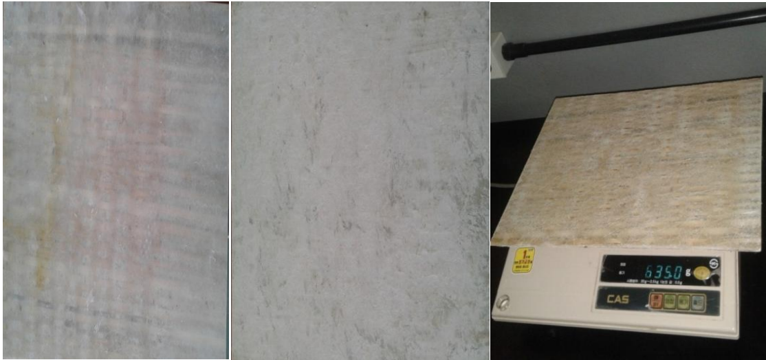
Figure 3.11: The final prepared mold for specimen in both sides and its weight
