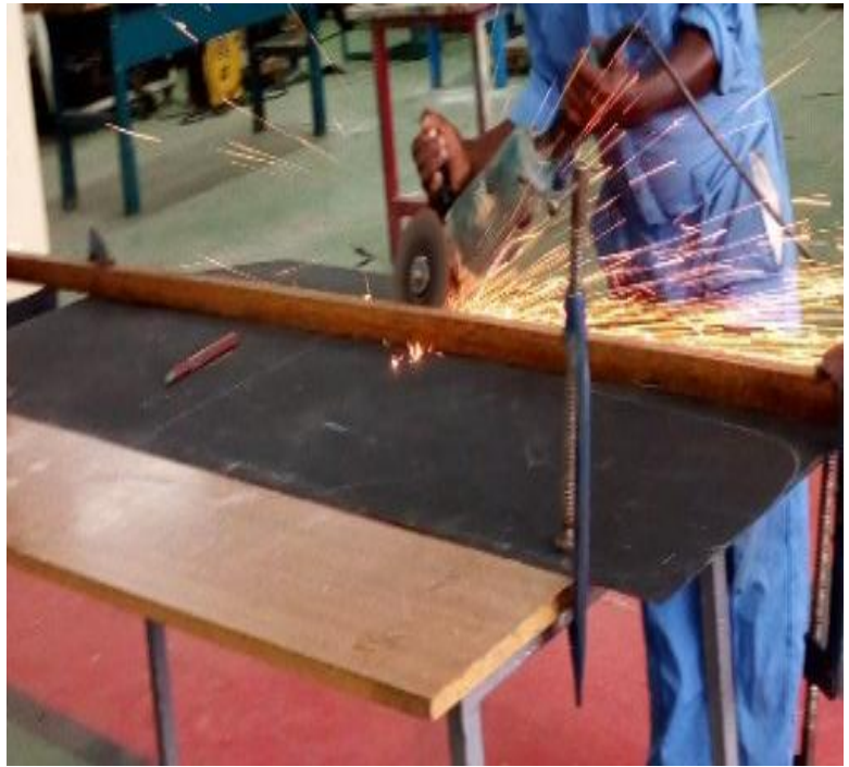
b). Cutting with grinding machine
