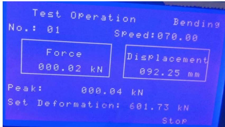
Figure 4.27: A1 90° fiber orientation flexural test
