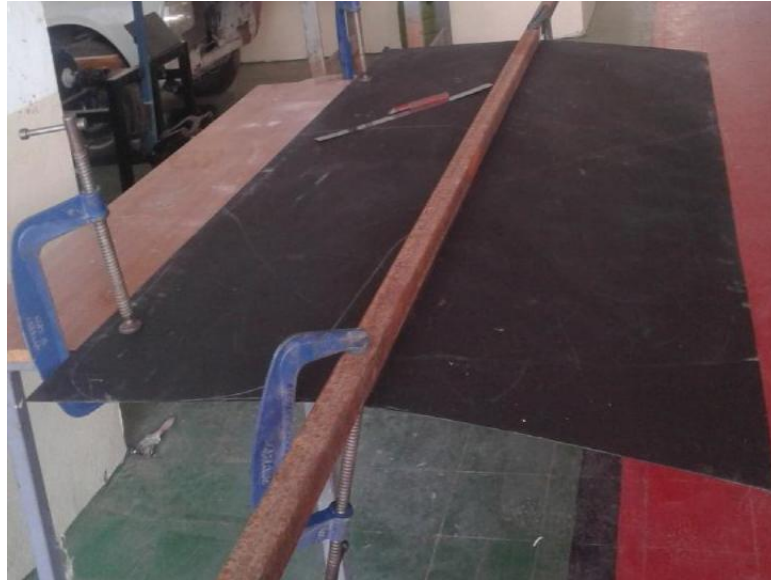
Figure A.1: fixing sheet metal on work bench
