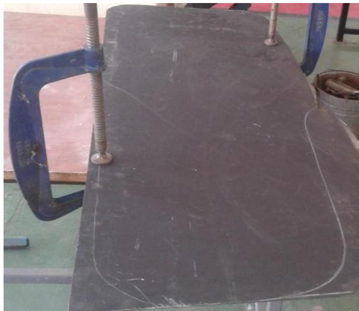
Figure A.2: Lines drawn on sheet metal
