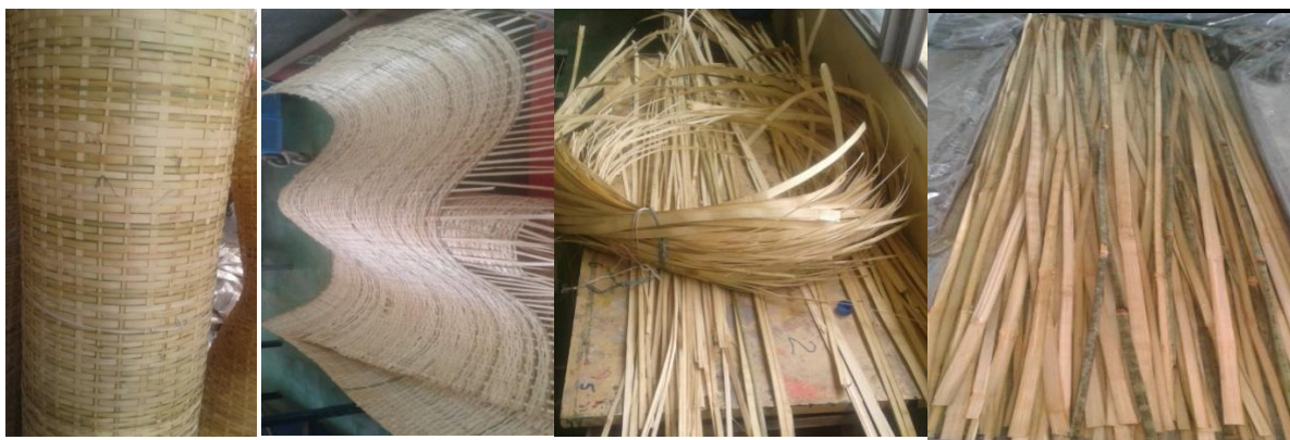
a).waved roll bamboo b). splitting process c). splinted bamboo d). final prepared bamboo strip
