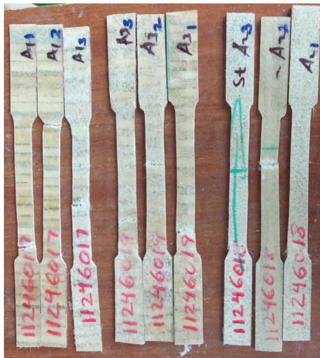
Figure 4.15: Tensile test specimen after test
