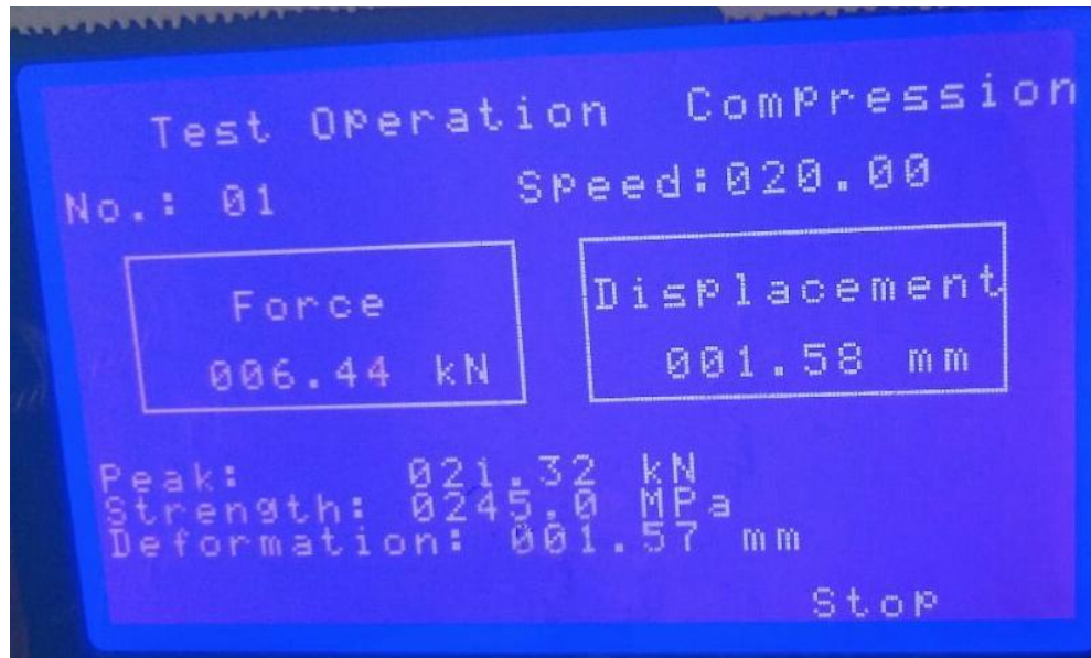
Figure 4.20: A2 (compression test for 0^0 fiber orientation)
