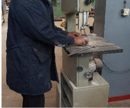
Figure 4.1: Test specimen preparation using Band Saw in AAiT
