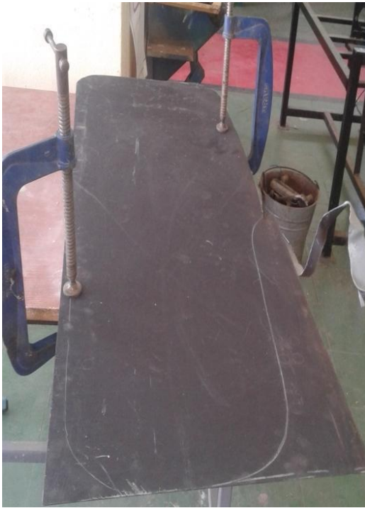
a). Marking sheet-metal with scissor
