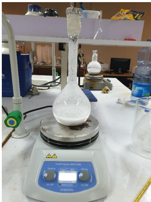
Figure 11. Impregnation of CaO by zinc doping
