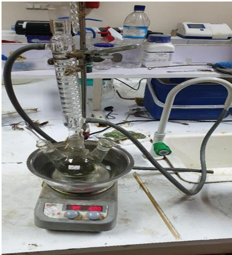
Figure 13. Experimental setup for transesterification reaction
