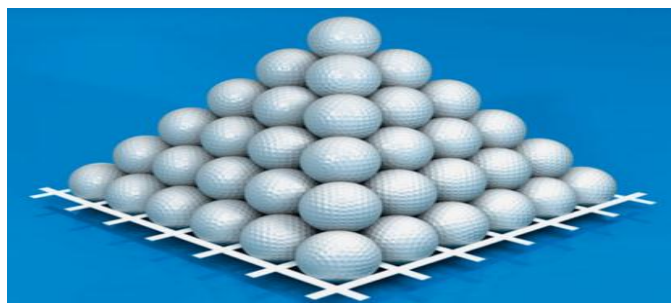
Figure 2.10 a geogrid an interlock with the soil aggregate [www.naue.com]
