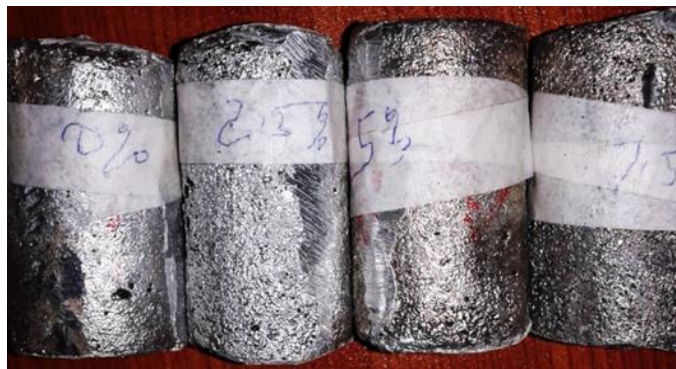
Figure 3. 10. Samples Perpared for Hardness Test befor Machining
