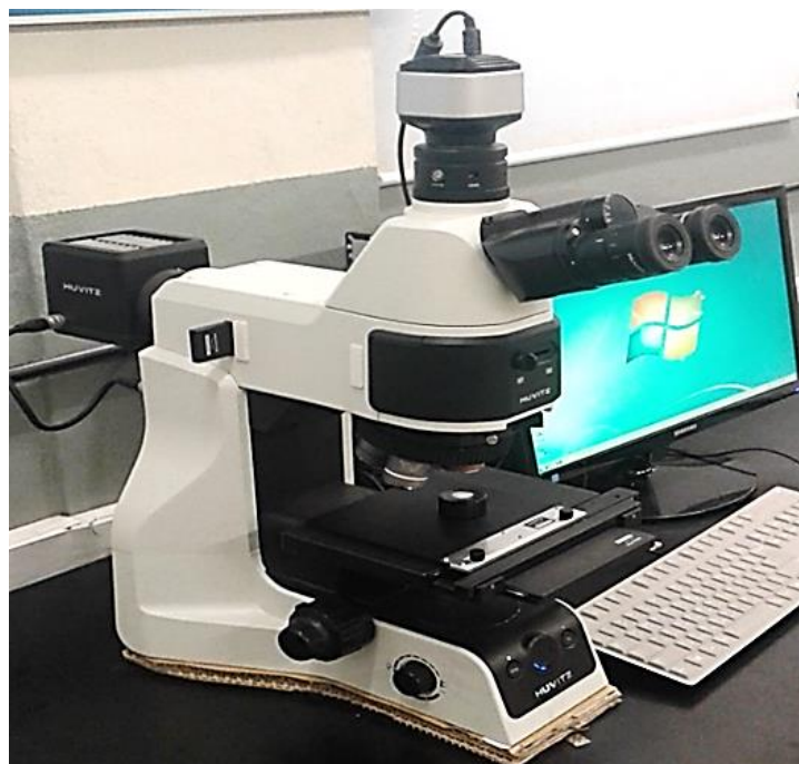
Figure 3. 15. Optical Microscope for Microstructure Study
