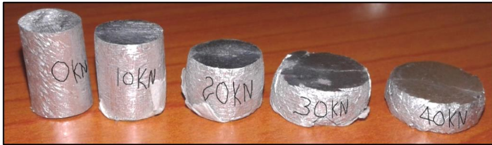
Figure 4. 10. Change of Specimen in Length and Diameter With Respect to Load
