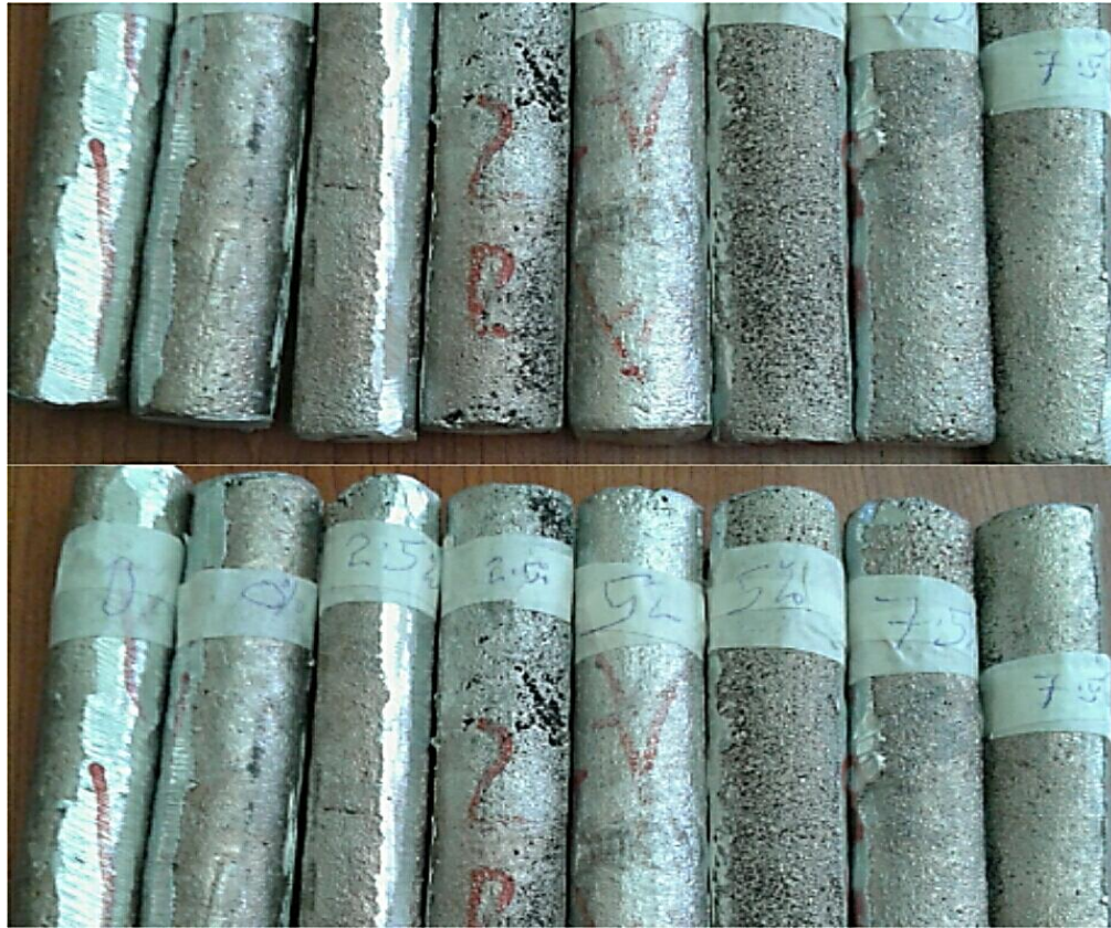
Figure 3. 7. Samples Prepared for Tensile Test before Machining
