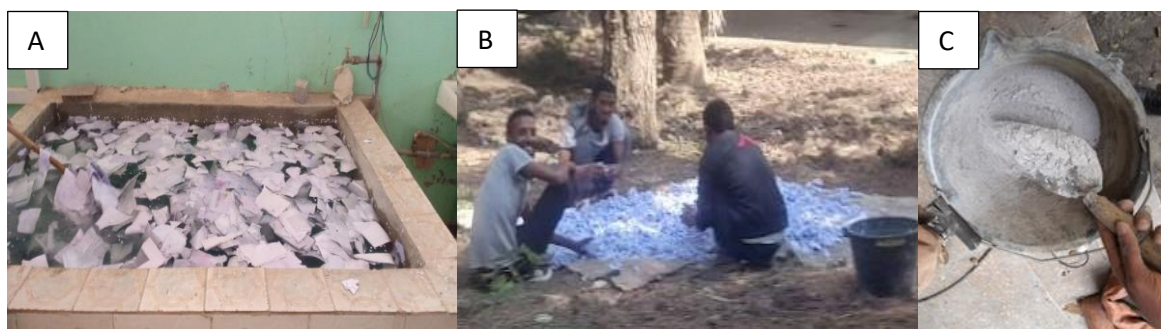
Figure 3.2 Shows the wet wastepaper, A, dried wastepaper, B, and wastepaper ash, C respectively.
