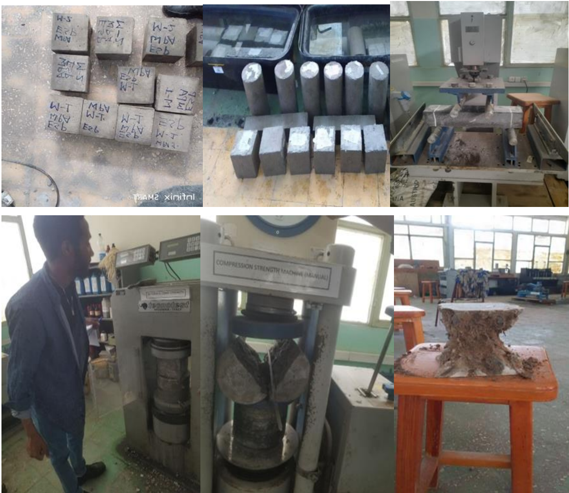
C1.4: Pictures captured during Curing and testing of concrete
