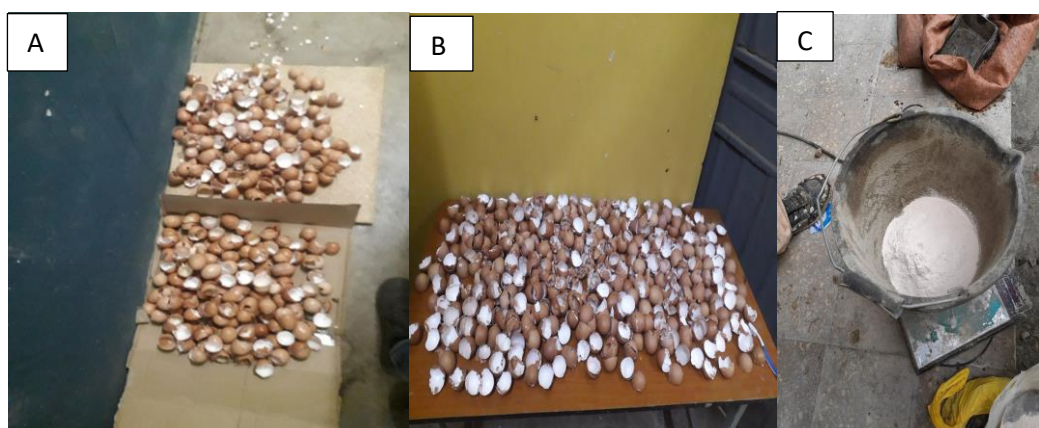
Figure 3.1 Shows the eggshell samples A, before wash, B, after washing, C, dried eggshell and eggshell powder respectively.
