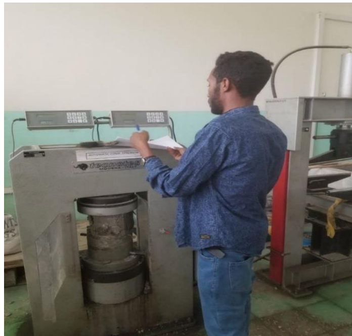
Figure 4.8 Compressive strength of concrete being tested.
