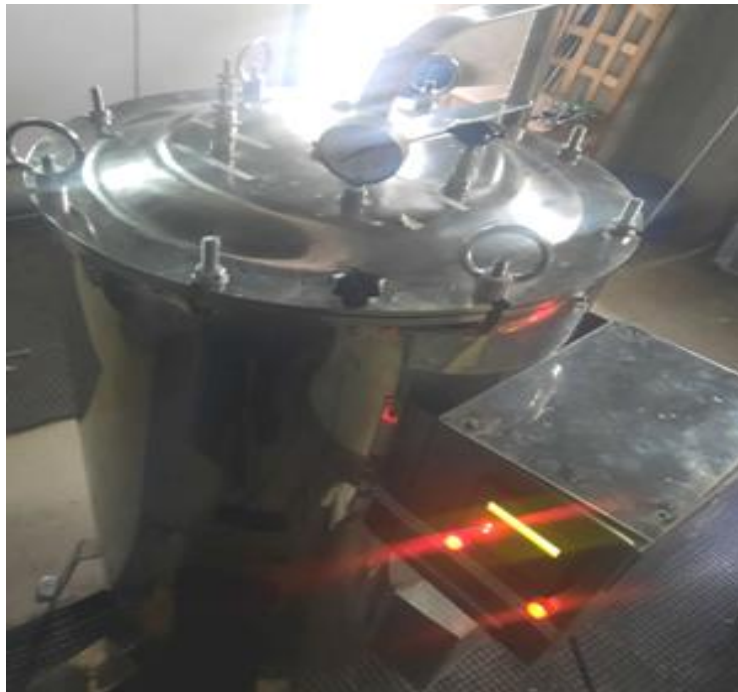
Figure 3.7: Construction of small-scale steam autoclave chamber (photo).
