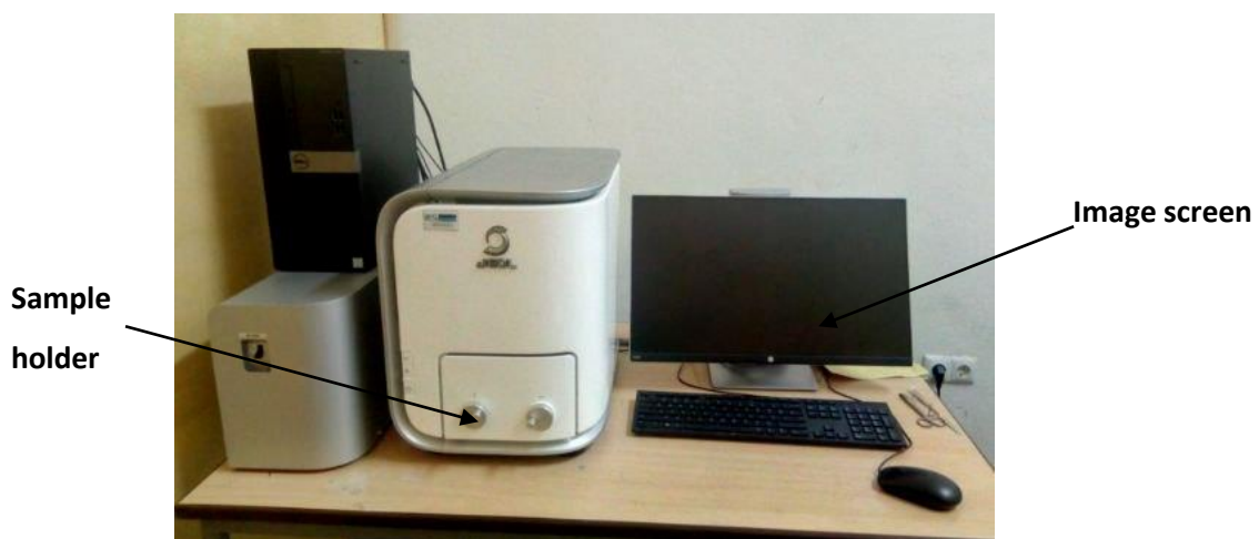
Figure 3.10: SEM for corrosion surface analysis (Photo).
