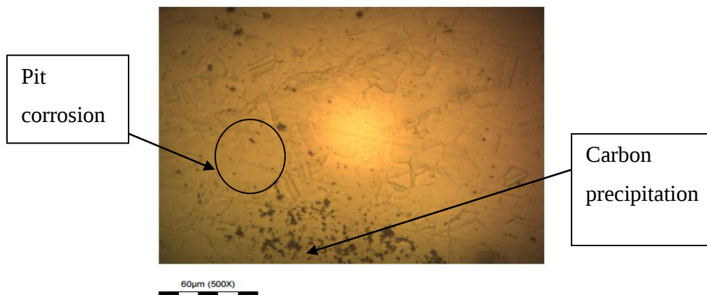
Figure 4.17: Image of metallographic of specimens after exposure to 3.5% \text{NaCl}_2 solution. Small Bright Spots shown on the figure revealed the presence of small, bright spots scattered across the surface of the samples. These localized areas of increased brightness are indicative of corrosion products or localized corrosion attack. The occurrence of these spots suggests that the protective passivation layer on the SS304 surface has been compromised, leading to the initiation of corrosion processes. This breach in the passive film allows for localized oxidation, resulting in the formation of bright spots which can be attributed to the accumulation of corrosion products such as iron oxides or hydroxides.
