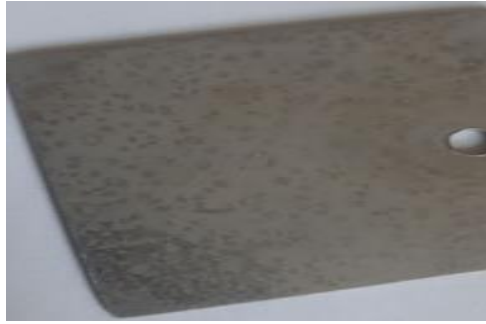
Figure 4.19: Image for samples exposed to 3.5%NaCl 2 solution for 336 hours(foto).
