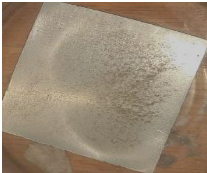
Figure 4.1: Sample of SS304 after exposed to 3.5%NaCl 2 solution for 120 hours before cleaning at room temperature (Photo).
