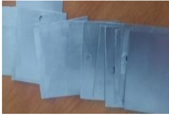
Figure 3.3: Prepared samples for immersion and exposure to steam autoclave (photo)
