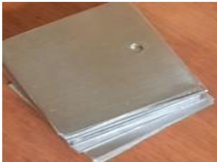
Figure 3.4: Samples prepared for exposure to steam autoclave conditions (Photo).
