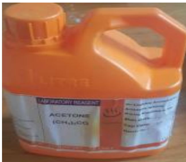
Figure 3.6: Acetone solution used to clean samples before and after exposure to the corrosive environment (photo).
