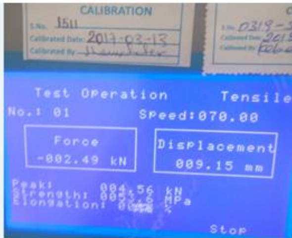
Tensile test result for natural bamboo (a) tensile strength (b) stress and strain curve
