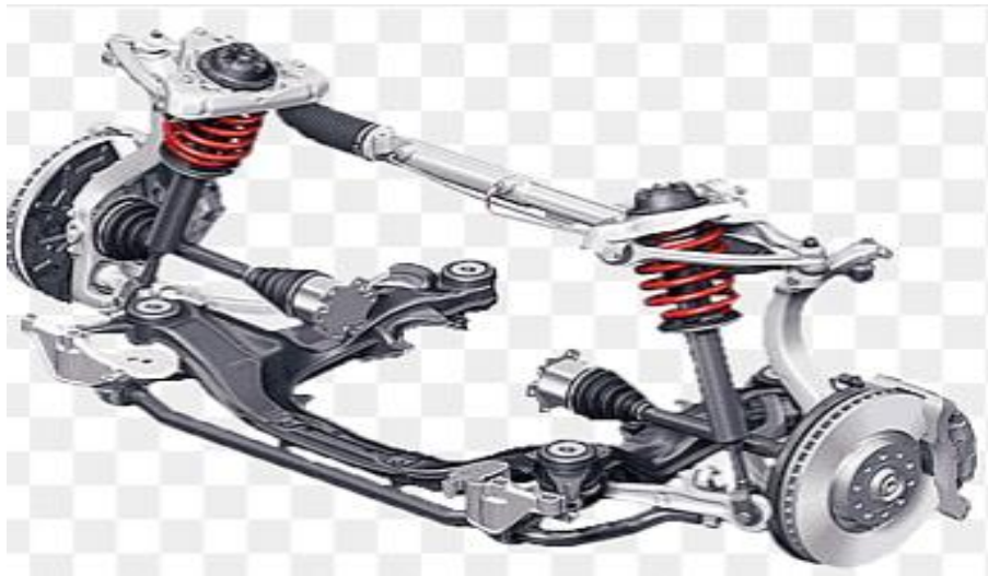
Figure 2.10: Double Wishbone suspensions (Julian Happian-Smith, 2002).
