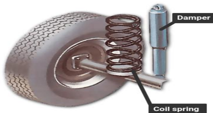
Figure 2.2: Damper (shock absorber) and Coil spring (Rudrakaanth et al., 2016).
