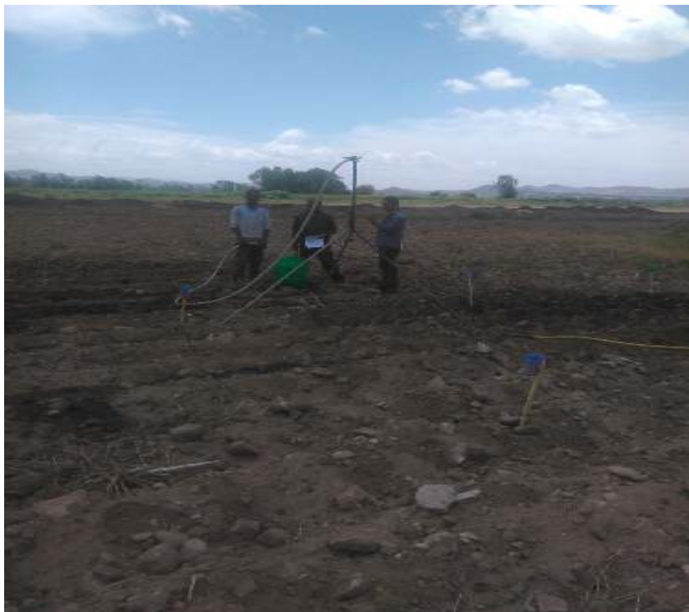
Appendix picture 1: Sprinkler discharge and water distribution measurements
