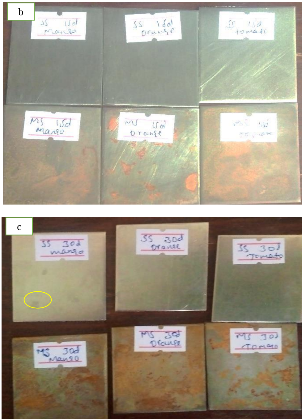
Figure 4.8 Image of corroded samples of stainless steel and mild steel; a) after 5 days exposure time, b) after 15 days exposure time and c) after 30 days of exposure time
