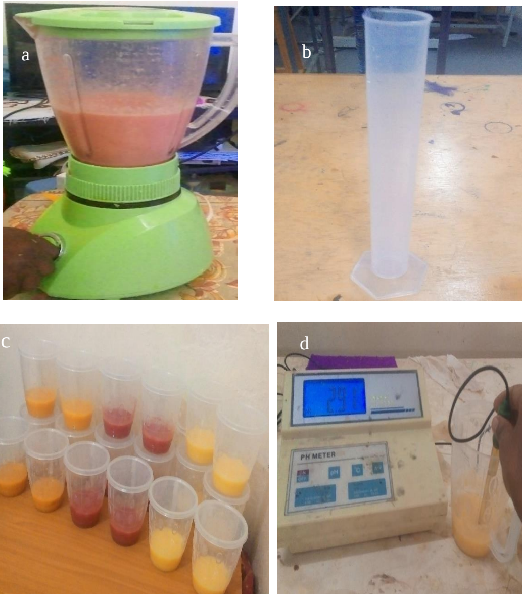
Figure 3.16 Experimental set-up: a) test solution preparation, b) test solution measurement, c) test solution in flask (beaker), d) pH measurement
