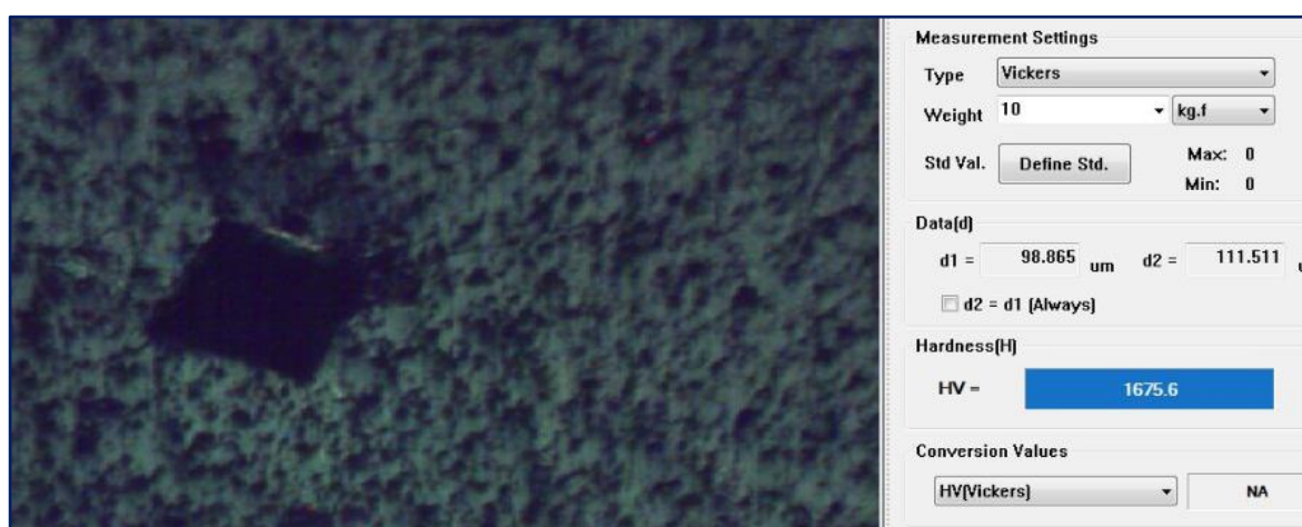
Figure B.4: Optical images of HEO pellet sintered at 1200 °C for 15 h.
