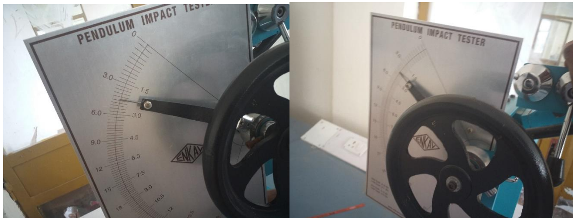
Adjustment and preparation of v -notch and, dial indicator after the load is applied
