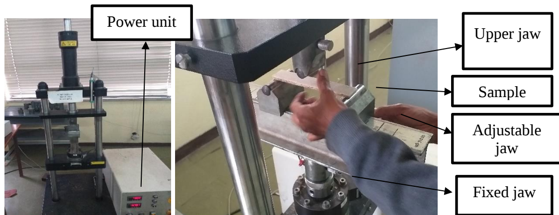
Figure 3.10 Universal Testing Machine for Flexural strength
