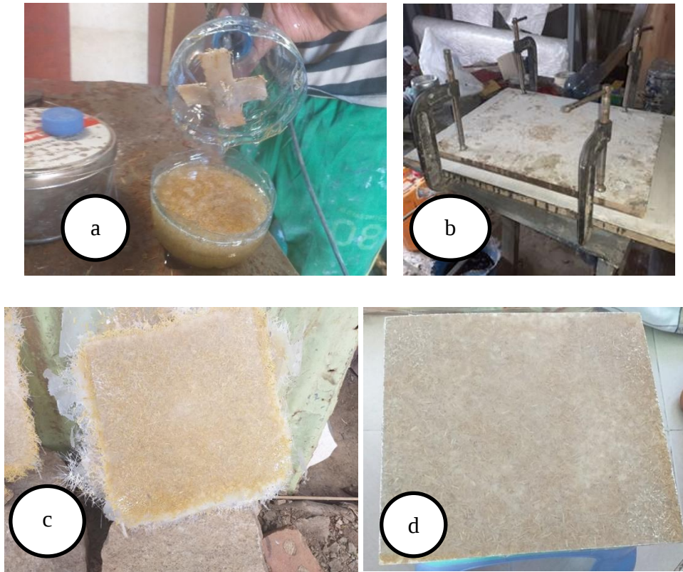
Figure 3.7 (a) Open mold and (b) stir casting (c) fabricated composite (d) fabricated composite with required size
