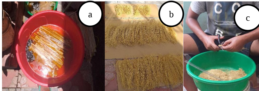
Figure 3.6 (a) Soaking of the bamboo fiber with NaOH (b) kept in sunlight (c) Cropped fibers
