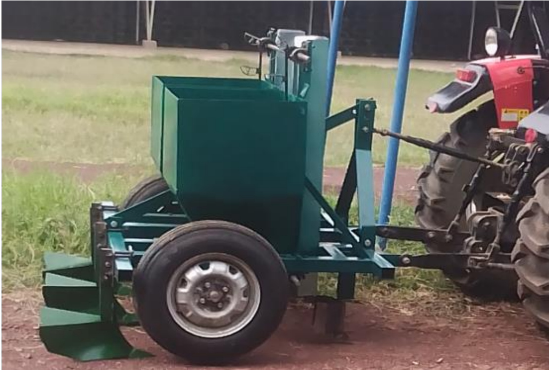
Fig 3.22. Fabrication pictures of tractor drawn potato planter
