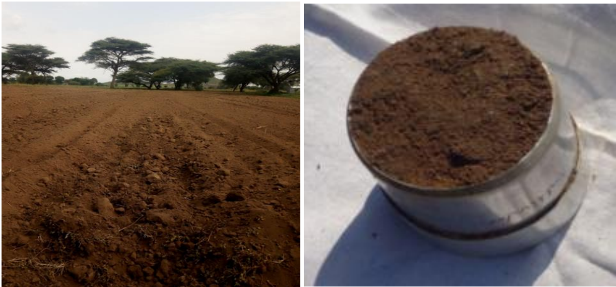
Fig 4.4. Measurement of soil density by core sampler
