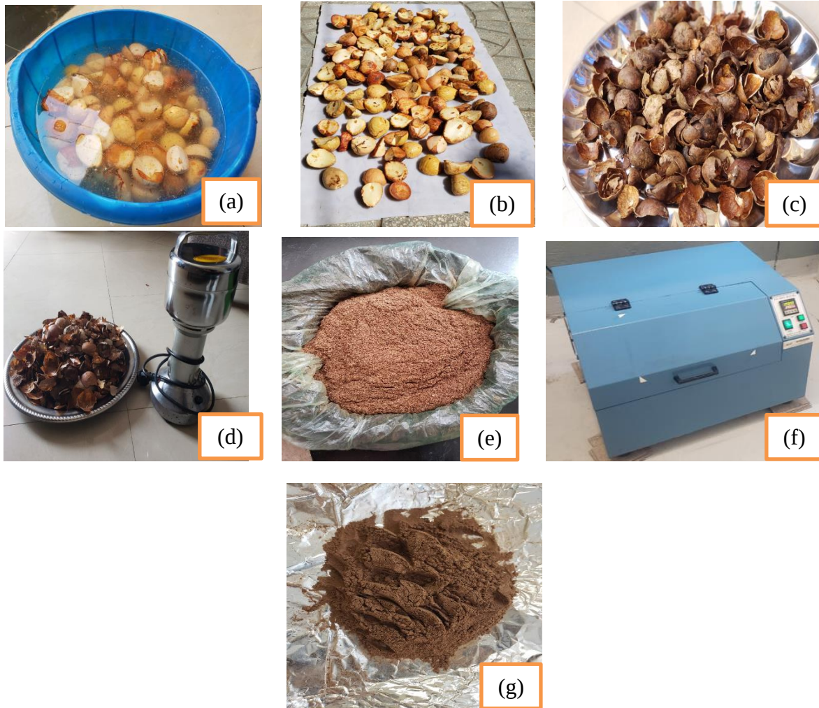
Figure 3.1: ASP preparation: (a): washed avocado seed, (b): drying the seed, (c): avocado cover peeled from the seed, (d): coffee grinder, (e): grinded ASP with coffee grinder, (f): ball milling machine, (g): milled ASP
