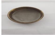
Figure 3.17: 75 microns size sieve
