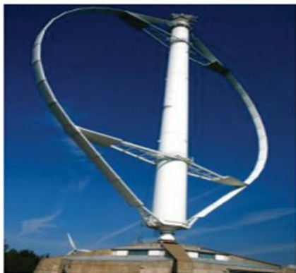
Figure 2-8: Darrieus wind turbines
